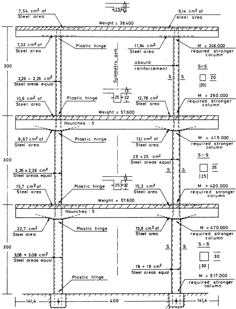
Fig. 1.- Left side was treated by the energy method. Right side was treated by the force method in which steel reinforcement results exaggerated in 1<sup>st</sup> and 2<sup>nd</sup> story; in 3<sup>rd</sup> story is absurd. Adopting the force method a stronger structure had been required, due to the lack of use of the structure ductility. Base of calculation:  $f_c = 84.4 \text{ Kg/cm}^2$ ;  $f_s = 2110 \text{ Kg/cm}^2$ ;  $n = 12$
