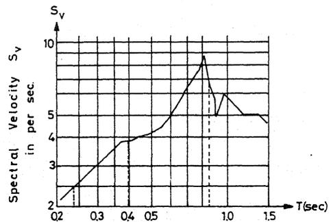
Fig. 5. Response spectra for elastoplastic systems with 10% critical damping,  $\mu = 4. (1)$
