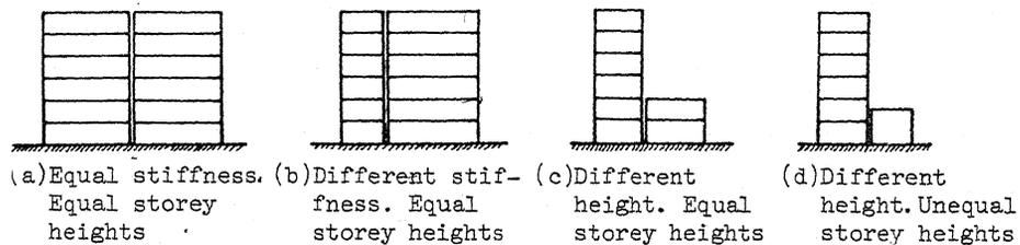
Fig.1 Structure to structure interaction
