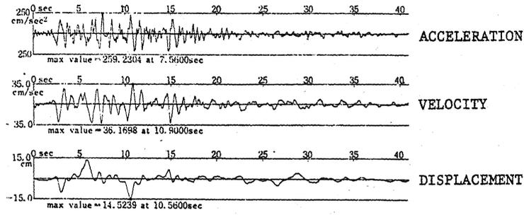
Fig.-5 Time Histories of Vibrations at Ground Level(N-S Component)
