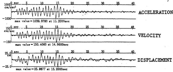
Fig.-6 Time Histories of Vibrations at 9th Floor(N-S Component)
