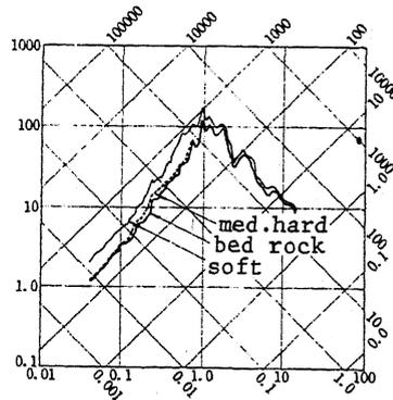
Fig.-10 Response Spectra for Fig.-9 in Tripartite. 5% damping
