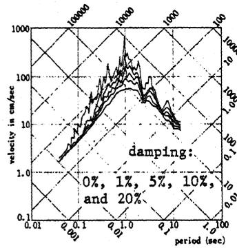
Fig.-8 Tripartite Response Spectra for Fig.-7
