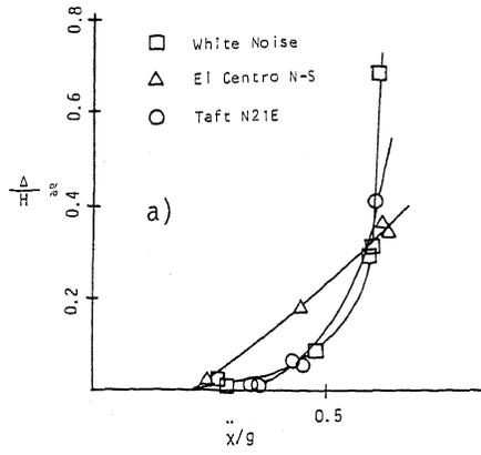
Figure 5. Permanent Displacement vs. Table Acceleration
