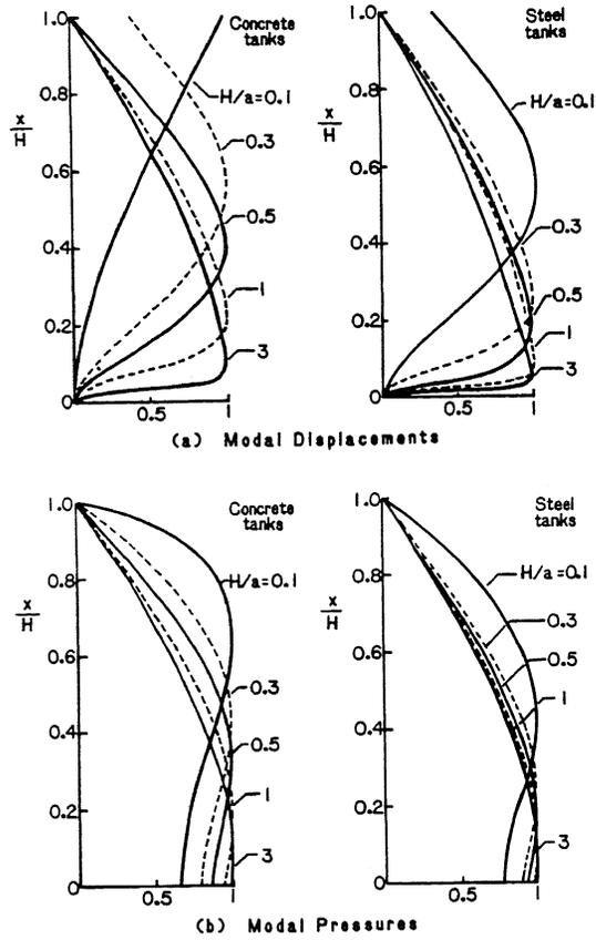
Fig. 1 Fundamental Modes of Axisymmetric Vibration of Liquid-Filled Tanks
