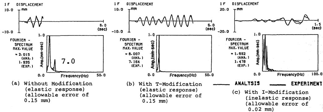
Fig. 10 Disp. Responses of 2 Story Steel Frame with Procedure Proposed
