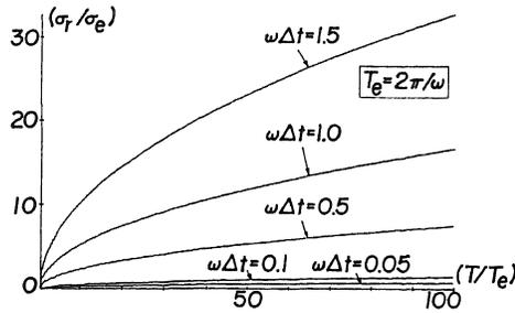
Fig. 7 Experimental Error Growth with Random Disp. Errors
