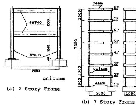
Fig. 9 2 and 7 Story Steel Frame Used in PSD Tests with Procedure Proposed
