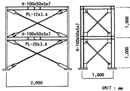
Fig.1 2 Story Steel Frame Used in PSD Test
