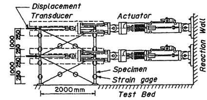
Fig.2 Test Setup Used for PSD Test
