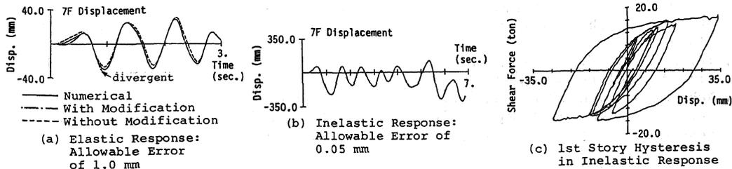
Fig. 11 Disp. Responses and Hysteresis of 7 Story Steel Frame with Procedure Proposed
