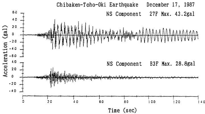
Fig. 5 Accelerograms on 3rd Basement and 27th floor
