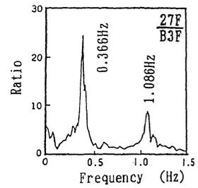
Fig. 6 Fourier Spectrum Ratio of Earthquake Motions in NS Direction
