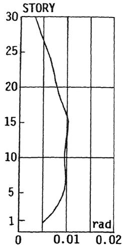
Fig.11 Max. Story Drift Angle
