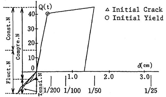
Fig.8 Analyzed Q- $\delta$  Curve of No.2 Specimen
