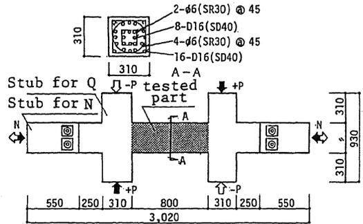
Fig.4 Structural Test Specimen of Column with Core Rebars
