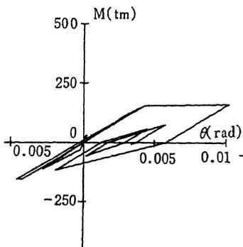
Fig.14 M- $\theta$  Hysteresis Loop at Beam End on the 15th Floor
