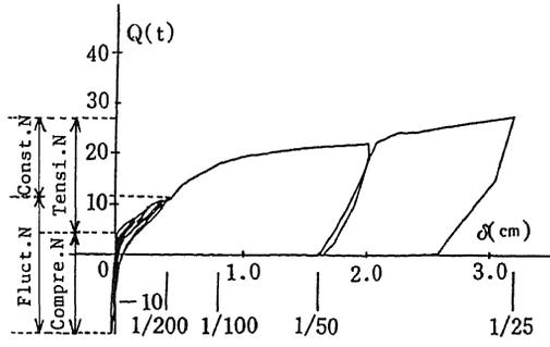
Fig.5 Tested Q- $\delta$  Curve of No.1 Specimen
