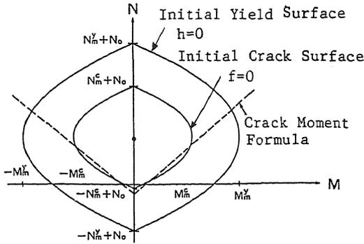
Fig.1 Initial Crack and Yield Surfaces
