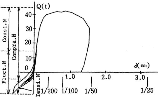
Fig.7 Tested Q- $\delta$  Curve of No.2 Specimen
