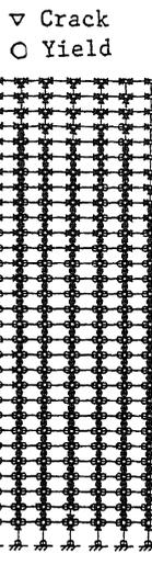
Fig.10 Occurrence of Crack and Yield after EQ.
