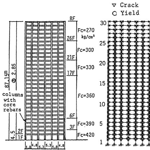
Fig.9 Analytical Object of a RC Frame
