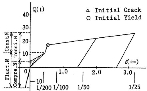
Fig.6 Analyzed Q- $\delta$  Curve of No.1 Specimen
