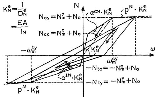
Fig.3 Assumed Uniaxial N- $\omega$  Hysteresis Loop
