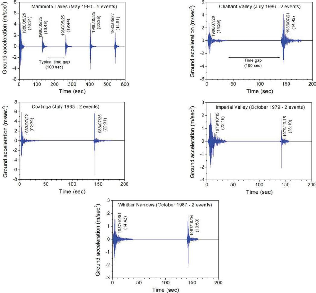
Figure 3. Ground acceleration records of the examined seismic sequences
