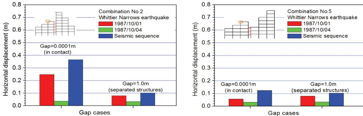
**Figure 7.** Max. horizontal top displacement of Frame F2 for pounding combinations No. 2 and 5.
