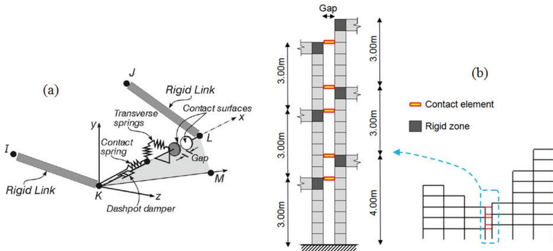
Figure 1. a) Ruaumoko contact element (Carr 2008), b) Modelling of structures interface
