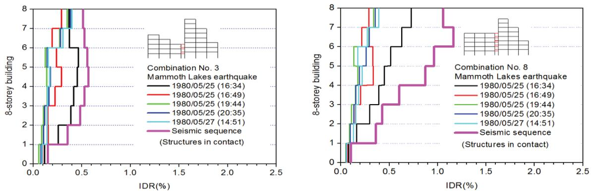
**Figure 8.** *IDR* diagram of pounding combination No. 3 and 8 – Structures in contact
