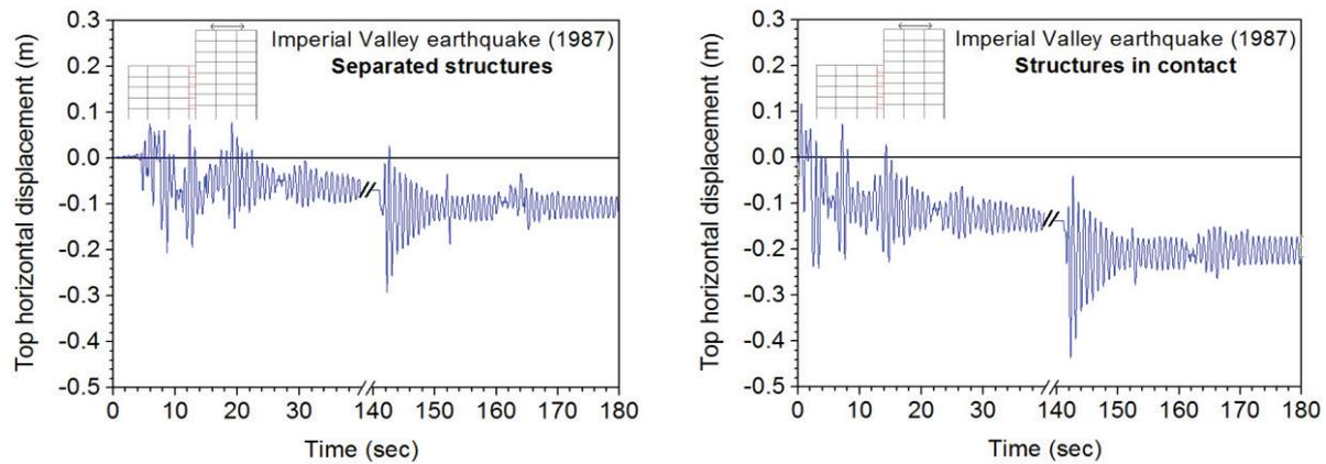
**Figure 9.** Top displacement time-history of the 8-storey frame (Comb. No. 1)
