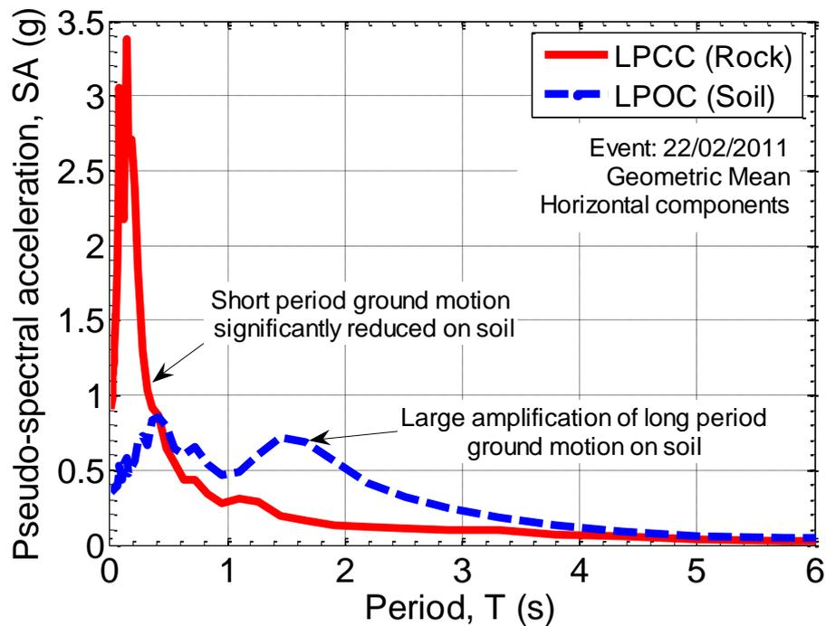
**Figure 7.1.** Comparison of the (geometric mean) horizontal ground motion response spectra at Lyttelton Port during the 22 February 2011 earthquake illustrating the importance of surficial soil response.
