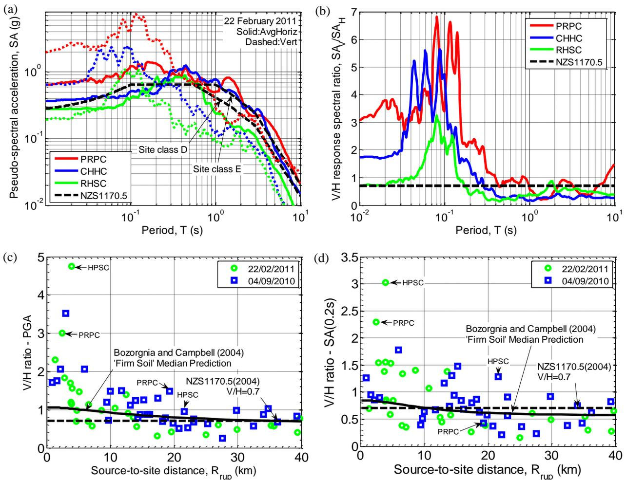
**Figure 8.1.** Vertical ground motion response spectral amplitudes observed: (a)-(b) Example geometric mean horizontal and vertical response spectra and their vertical-to-horizontal ratio; (c)-(d) vertical-to-horizontal response spectral ratios for  $T = 0.0$  and  $0.2$ s as a function of distance observed in the 4 September 2010 Darfield and 22 February 2011 Christchurch earthquakes and comparison with the empirical prediction of Bozorgnia and Campbell (2004).
