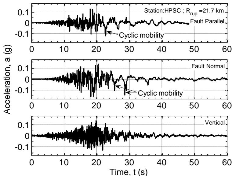
**Figure 7.2.** Evidence of liquefaction in the form of cyclic mobility in the acceleration time history recorded at Hulverstone Drive (HPSC) during the 22/02/2011 Christchurch earthquake.
