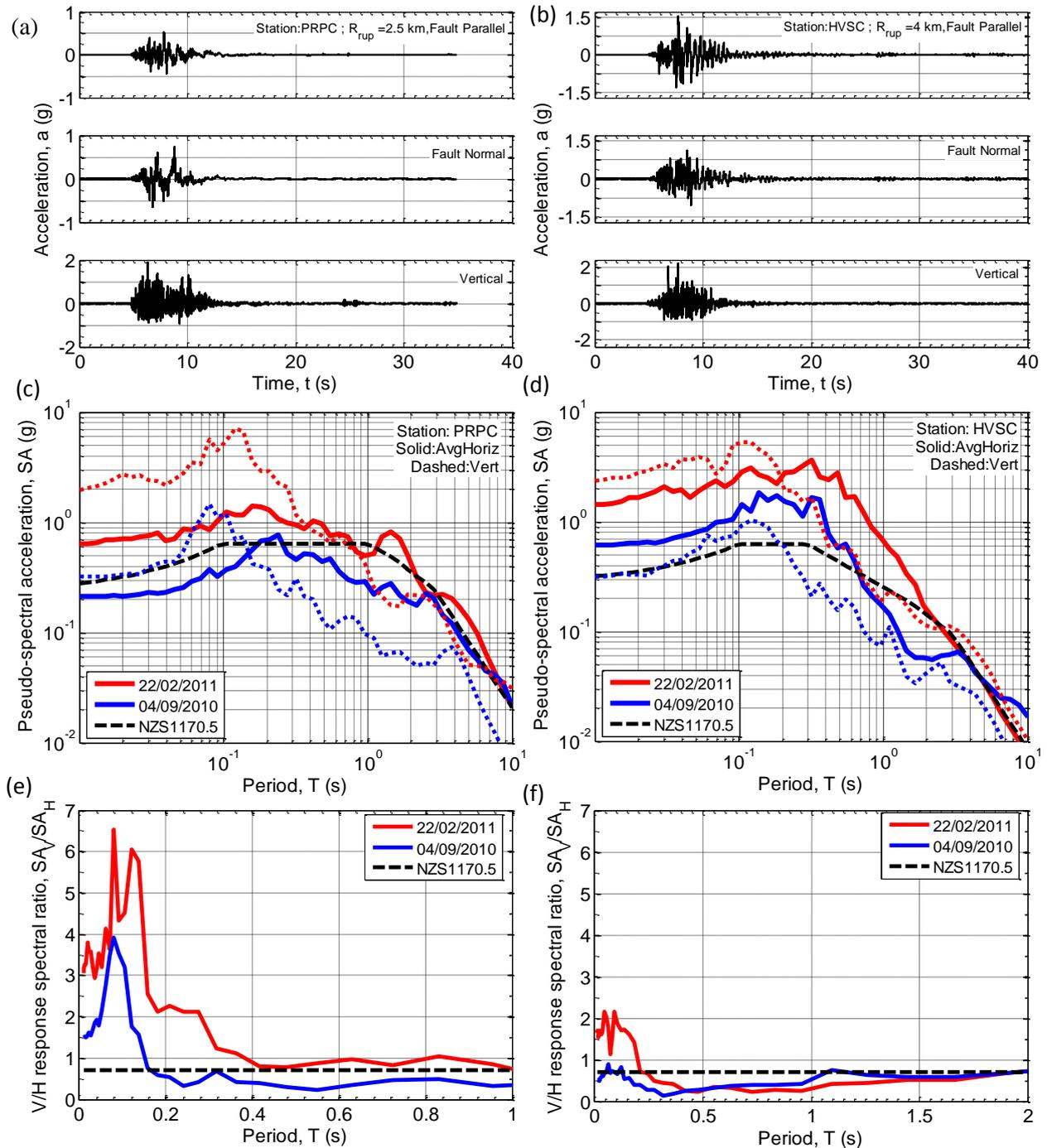
**Figure 3.1.** Extreme ground motions observed at Pages Road (PRPC) and Heathcote Valley (HVSC) in the 22 February 2011 Christchurch earthquake in terms of acceleration time history, pseudo-acceleration response spectra, and vertical to horizontal spectral ratios. Note the different scale used for vertical acceleration time histories in Figure 3.1a and Figure 3.1b with that of the horizontal.
