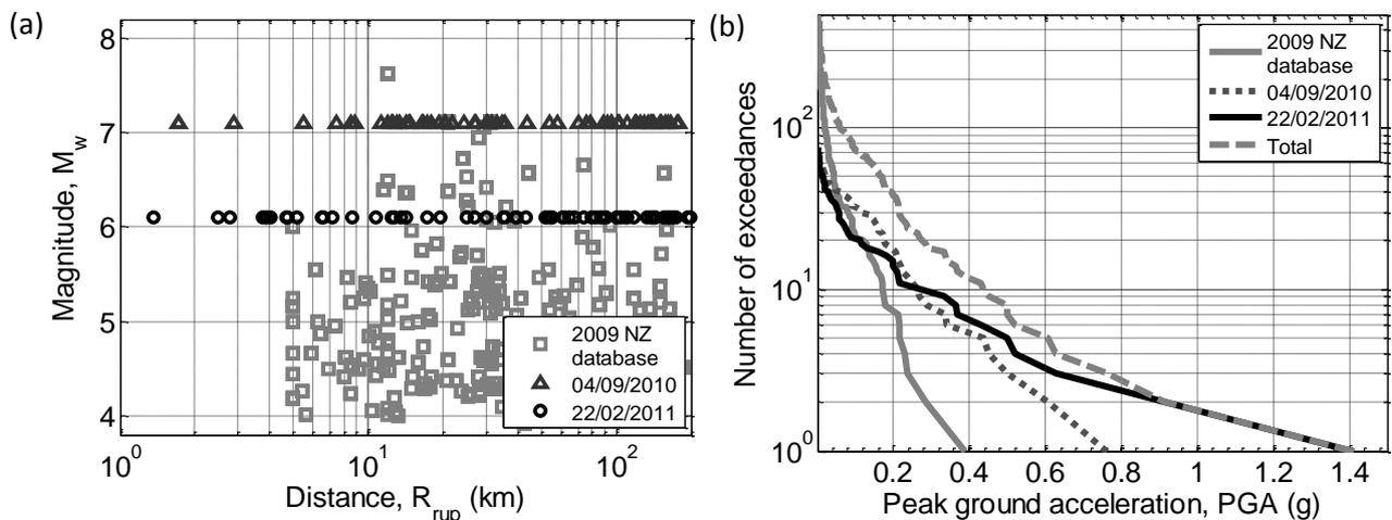
**Figure 2.1.** Significance of the 22/02/2011 Christchurch and 04/09/2010 Darfield earthquakes in relation to previously recorded ground motions in New Zealand: (a) magnitude-distance distribution; (b) exceeded values of peak ground acceleration.
