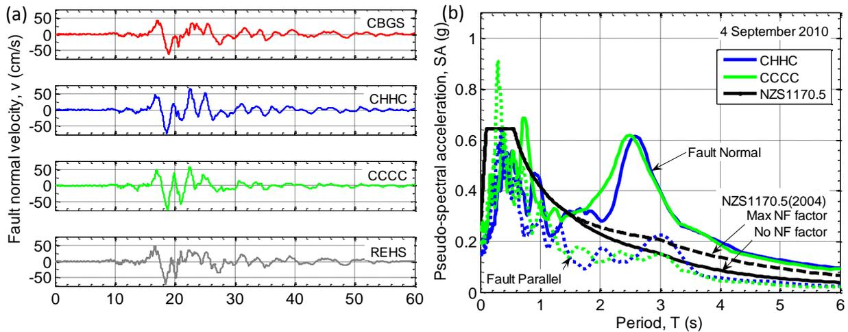
**Figure 4.2.** Forward directivity effects observed in the Christchurch central business district (CBD) resulting from the 4 September 2010 earthquake: (a) fault normal velocity time series; and (b) fault normal (plain) and fault parallel (dashed) response spectra in comparison with those prescribed by NZS1170.5:2004.
