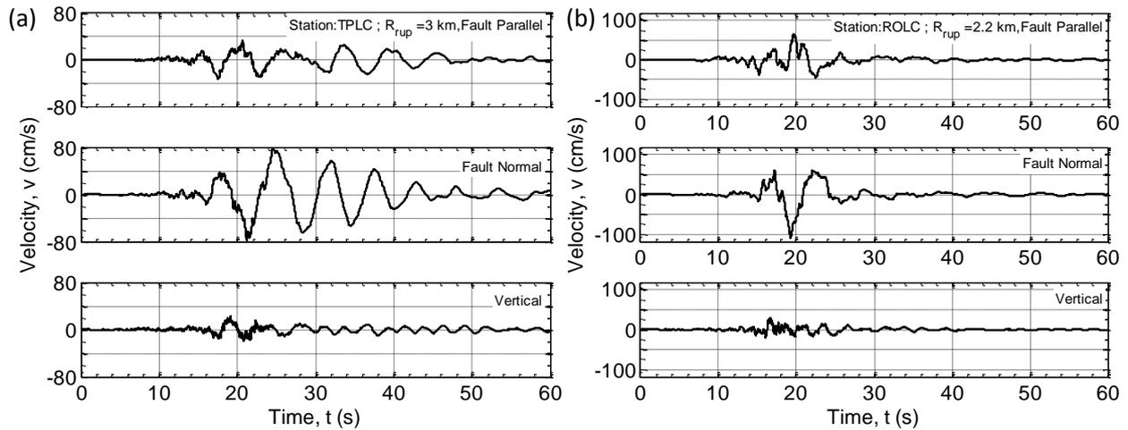
**Figure 4.1.** Evidence of strong forward directivity effects at locations to the east of the Greendale fault: (a) Templeton (TPLC); and (b) Rolleston (ROLC) resulting from the 4 September 2010 earthquake.
