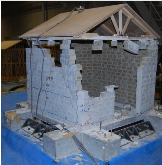
Figure 3.1.10: Door side photo after run 45 (5HZ-0.6g) of experiment (Sathiparan, N. 2008)
