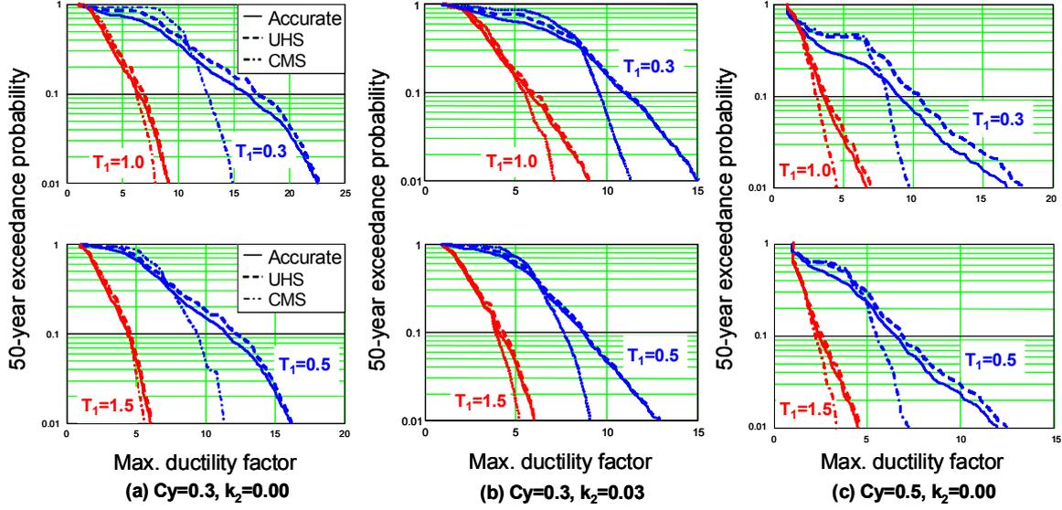
**Figure 4.** The exceedance probability of  $S_{D50}^I$  estimated by the CS method using a UHS or a CMS
