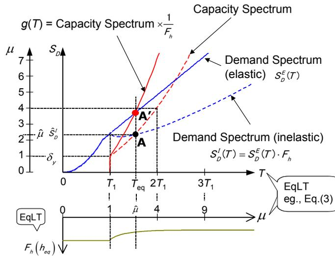
Figure 1. Capacity spectrum method in  $T-S_D$  coordinate
