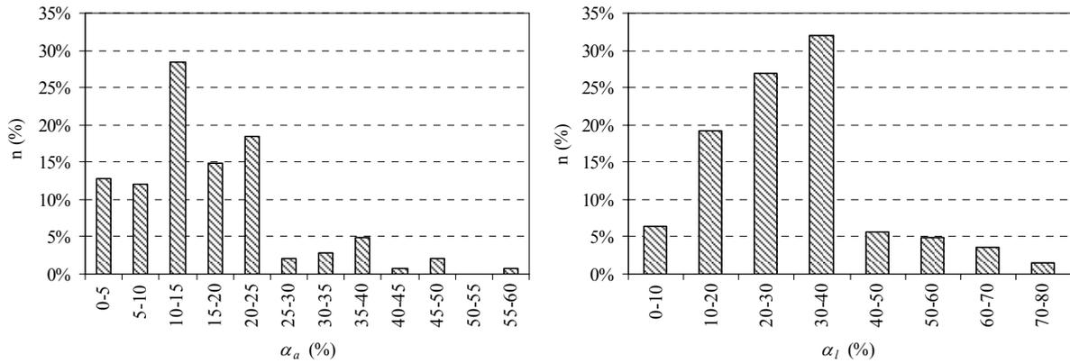
**Figure 3.1.** Distribution of tests according to the opening dimensions.
