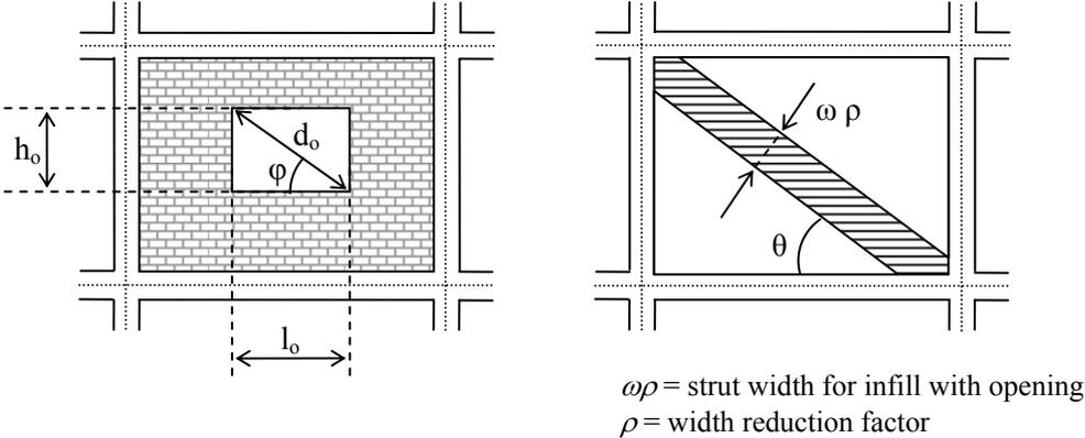
**Figure 2.2.** Diagonal strut model for infill with opening.
