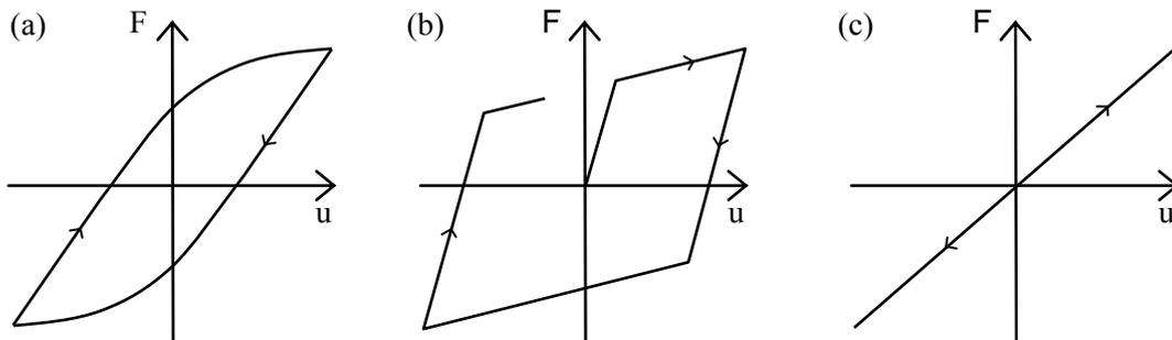
**Figure 2.1:** Typical force-displacement characteristics for the (a) Bouc-Wen, (b) bilinear and (c) linear models.
