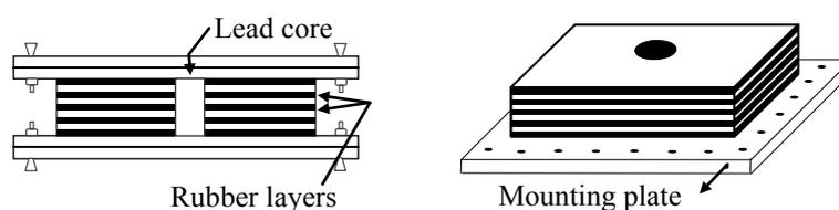
**Figure 1.1:** Lead Rubber Bearings.
