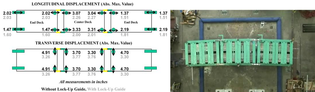
(a) Plan view of isolation bearing displacements (b) Maximum transverse response with lock-up guide
