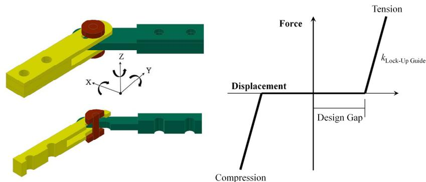
(a) Isometric AutoCAD sketch-up (b) Theoretical longitudinal force-disp. relationship
