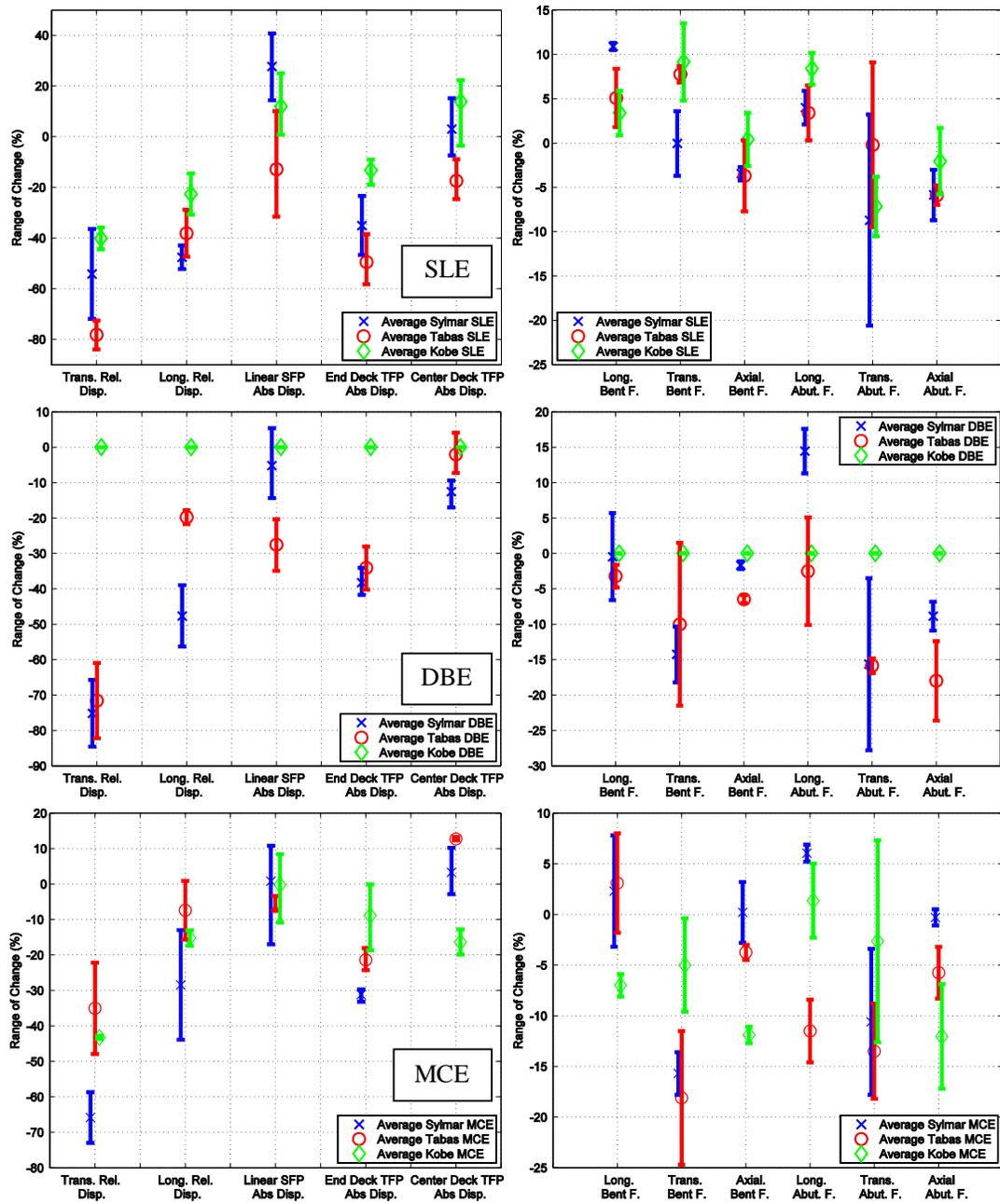
**Figure 4.1.** Displacement and force comparison between isolated bridge with and without Lock-Up Guide Set#2 at SLE, DBE, and MCE excitation levels
