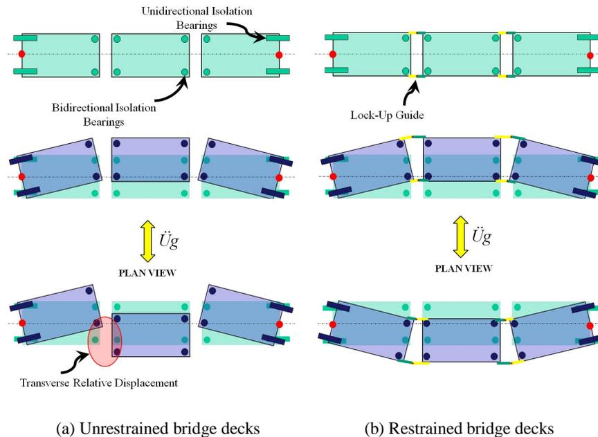
**Figure 2.1.** Segmental displacement control design concept plan view
