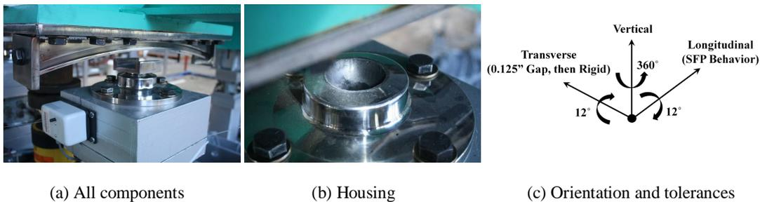
**Figure 3.2.** Experimental concave SFP isolation bearing
