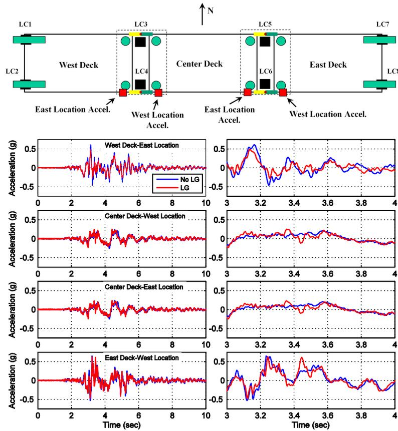
Figure 4.4. Superstructure accelerometer deck locations and time histories
