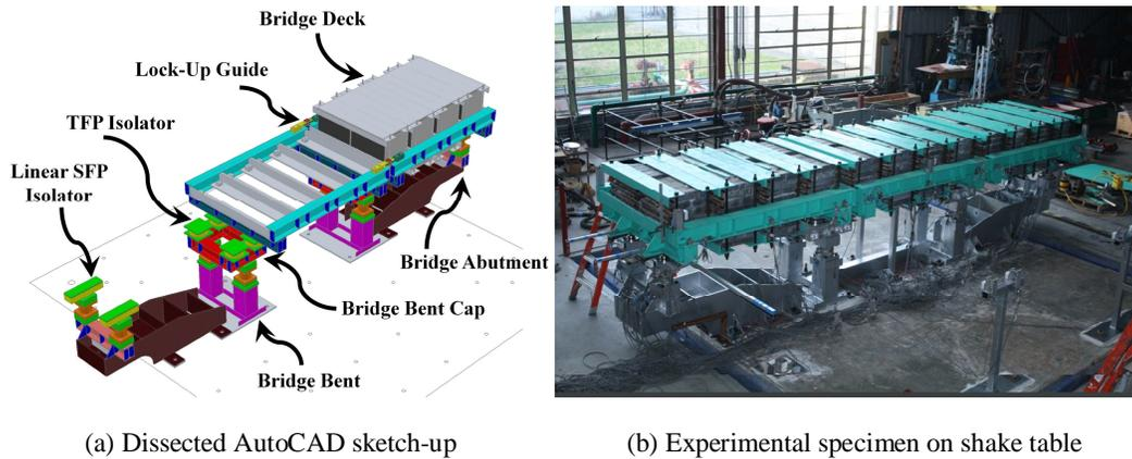
**Figure 3.1.** Quarter-Scale Isolated Bridge
