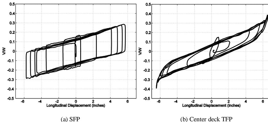
Figure 3.4. Normalized force displacement hysteresis of isolation bearings
