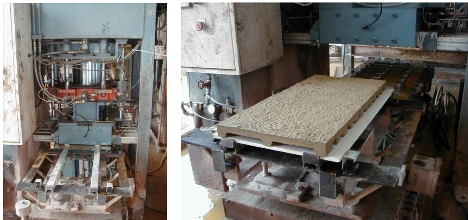
Photograph 3. The manufacture situation of PCa panels by compacting machine
