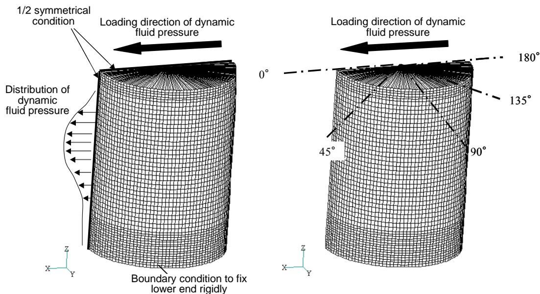
(a) Boundary condition of analysis model (b) Loading direction of dynamic fluid pressure
