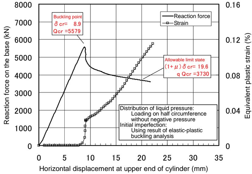
**Figure 4.5.** Load-displacement curve (FM-2)
