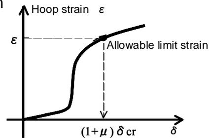
Estimation for allowable limit coefficient
