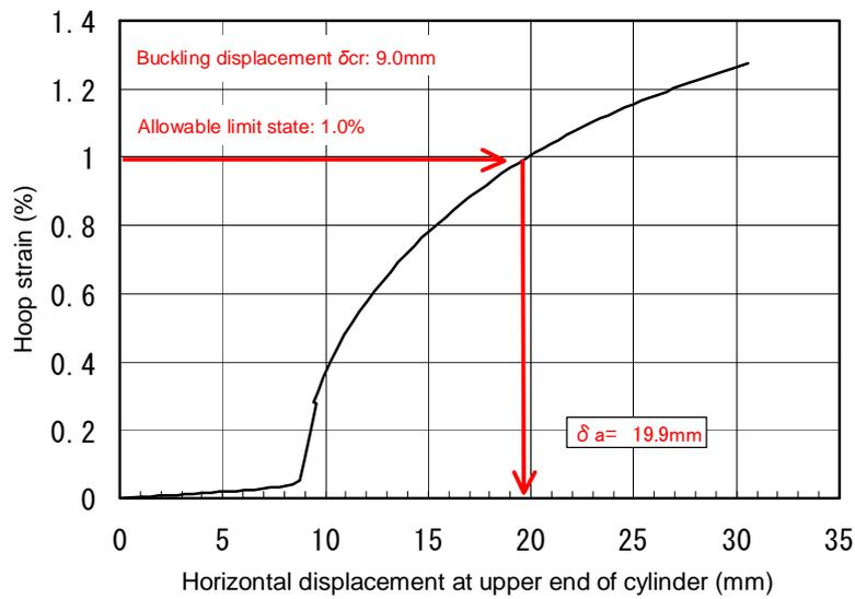
**Figure 4.4.** Hoop strain history at buckling position (FS-1)
