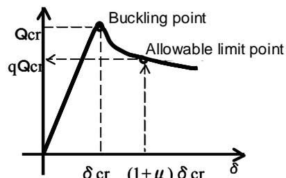
Estimation for coefficient to reduce loading capacity
