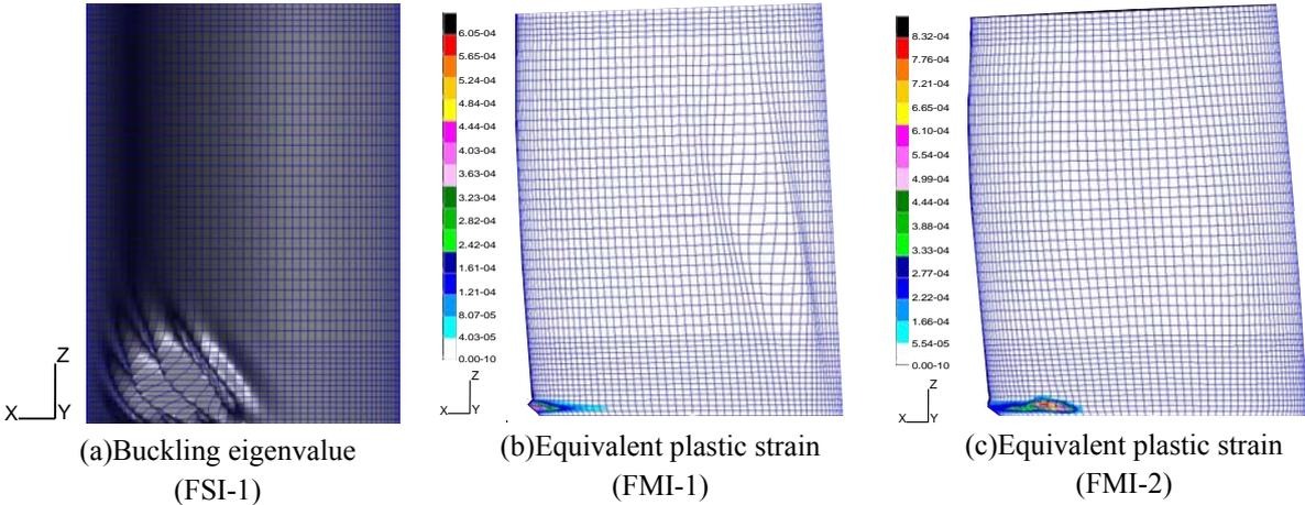
**Figure 4.1.** Results of elastic buckling analysis and elastic-plastic buckling analysis
