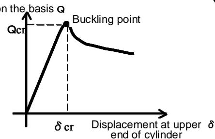
Acquisition of loading capacity characteristics
