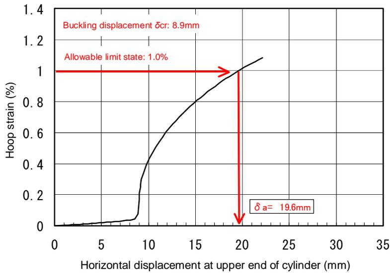
**Figure 4.7.** Hoop strain history at buckling position (FM-2)
