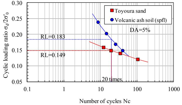
Figure 3. Comparison of liquefaction strength
