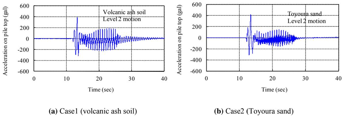
**Figure 8.** Response of acceleration on pile top
