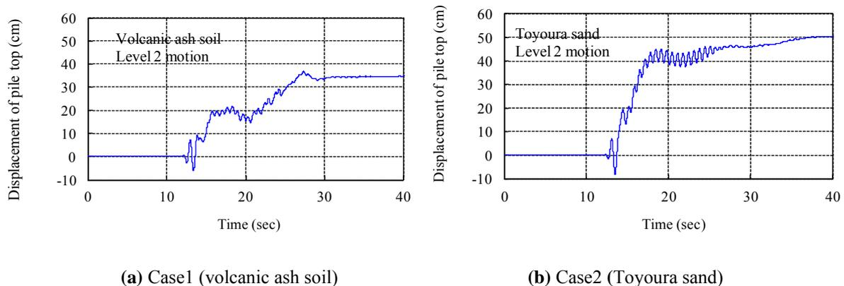
**Figure 9.** Response of displacement on pile top (measured by laser displacement gauge)
