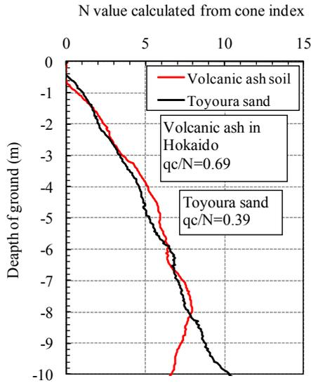
Figure 2. Results of cone penetration tests
