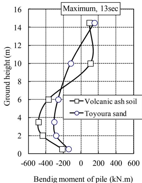
**Figure 11.** Maximum bending moment of pile in depth direction
