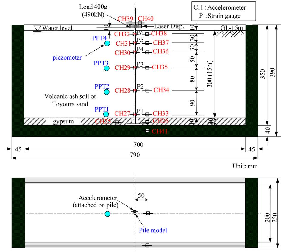
**Figure 1.** Outline of centrifuge model tests
