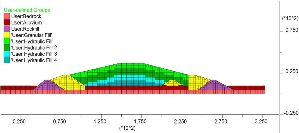
Figure 2.2. Finite Difference Grid
