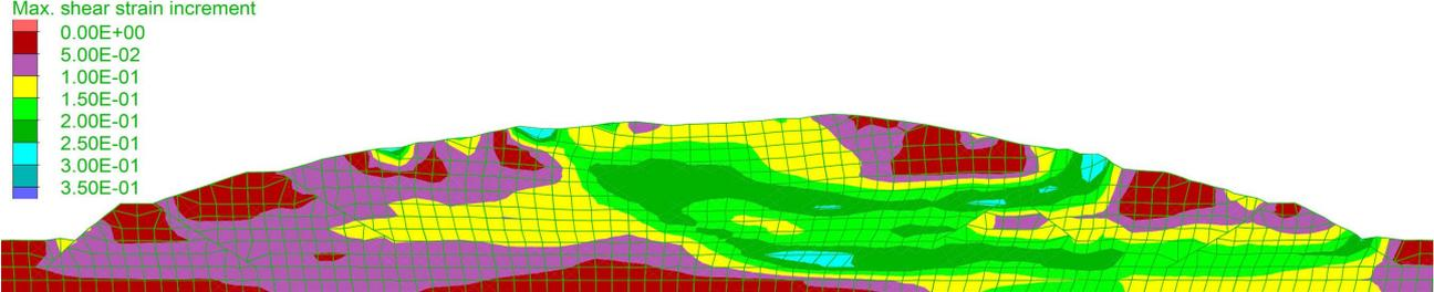
**Figure 3.6.** Plastic Shear Strains After Earthquake (MDE)
