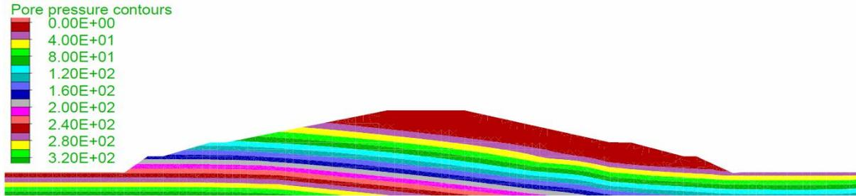
Figure 3.1. Initial Pore Water Pressure Distribution
