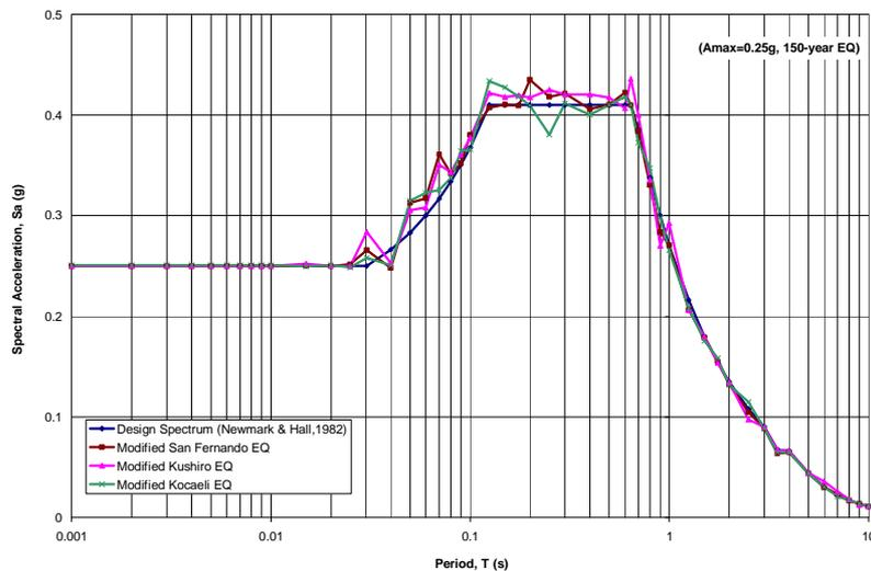
**Figure 2.4.** Acceleration Response Spectra of the Ground Motions (OBE)
