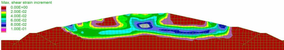
**Figure 3.3.** Plastic Shear Strains After Earthquake (OBE)
