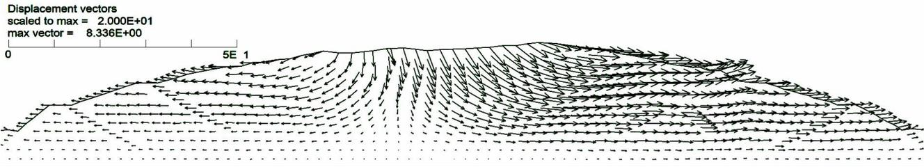
**Figure 3.5.** Permanent Deformation Vectors (MDE)
