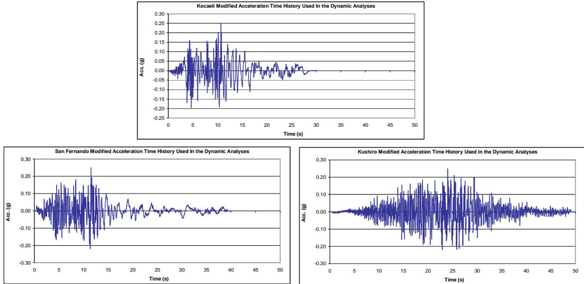
**Figure 2.3.** Acceleration-Time Histories Used in the Analyses (OBE)
