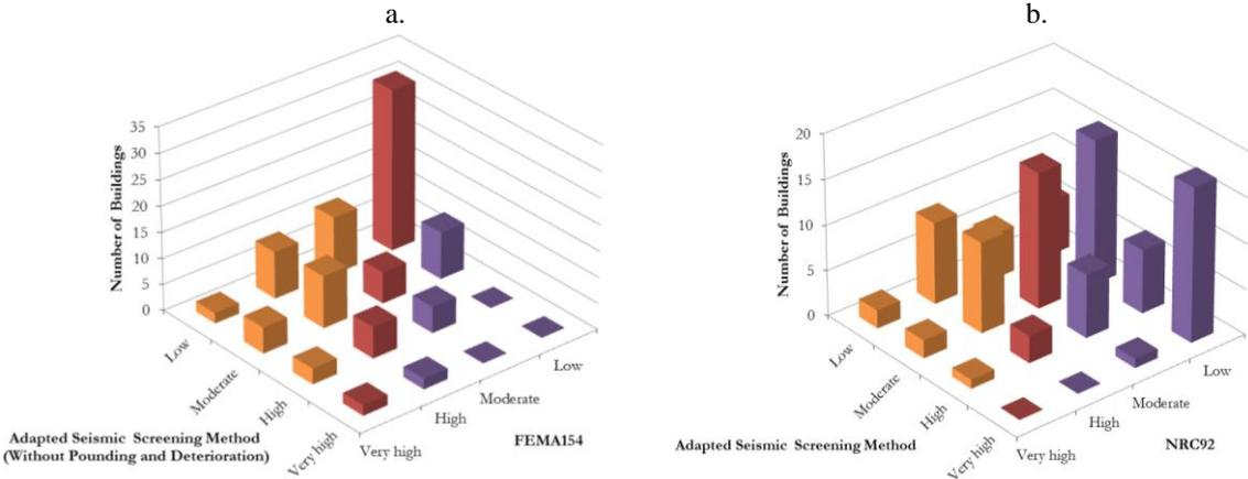
**Figure 6.1.** Distribution of building classification for the adapted seismic screening method compared to (a) FEMA154 and (b) NRC92
