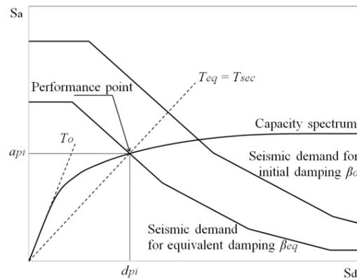
**Figure 2.1.** Capacity spectrum method, adapted from (ATC, 2005)
