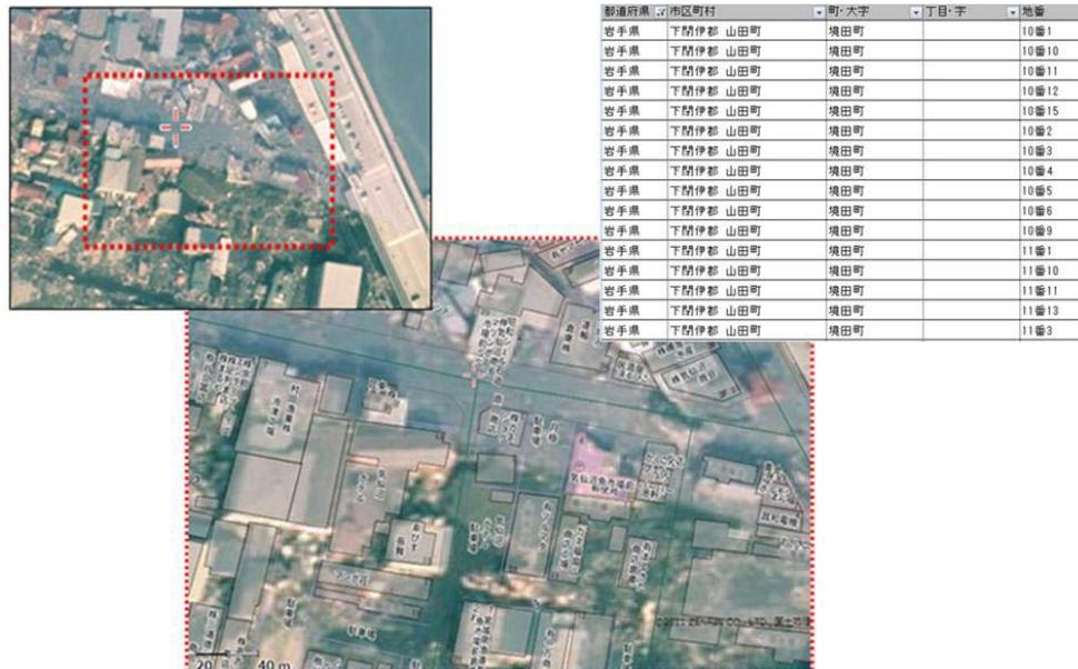
**Figure 16.** Post-tsunami aerial photograph taken by GSI (top left), same aerial photograph overlaid with Zenrin (2011) footprint dataset (middle) and list of addresses of structures recognised by SONPO (2011) to have been washed away by the tsunami (top right).
