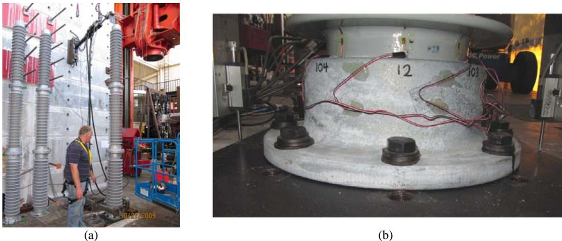
**Figure 7.** Setup for strain gage calibration (a) and zoomed view of the bottom part with two position transducers accounting for flexibility of the attachment if any (b)
