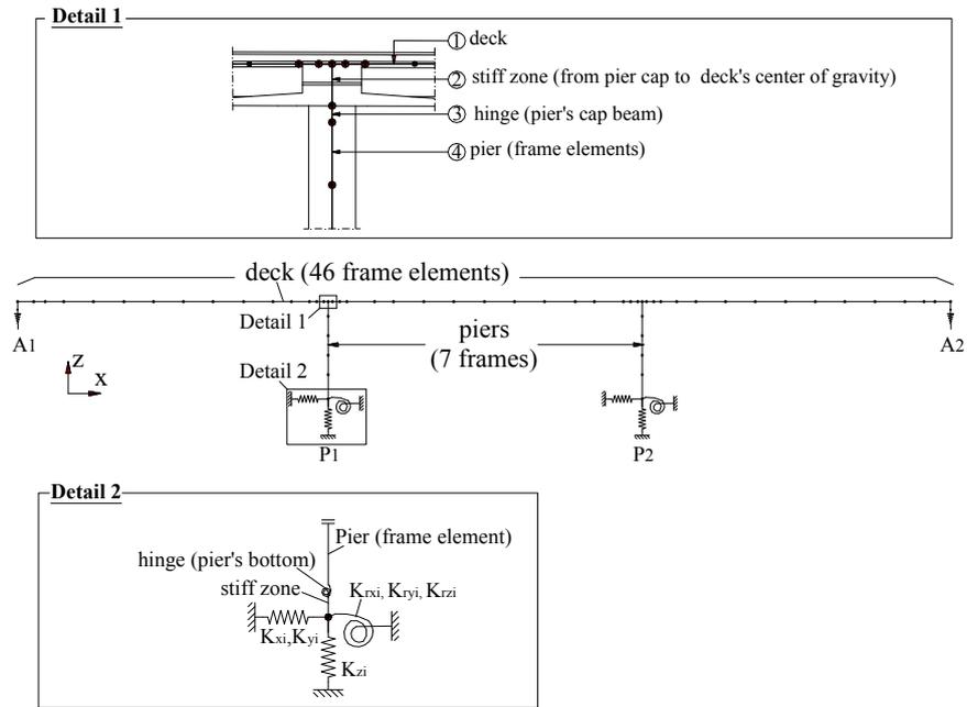
**Figure 4.** The stick model of Kleidi-Kouloura bridge without abutment-backfill participation, **Detail 1:** Modeling of the monolithic deck to pier connection, **Detail 2:** Modeling of the foundation and the possible hinge of the pier's bottom.
