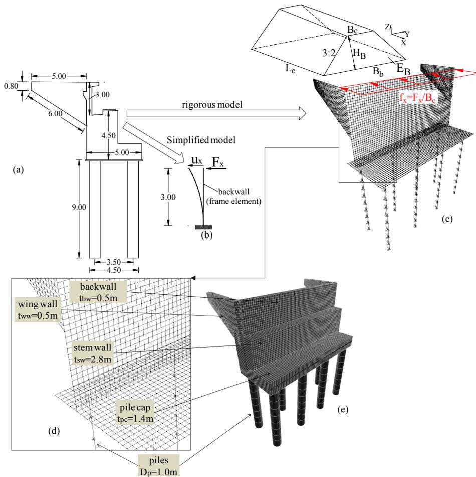
**Figure 5.** (a) Longitudinal section of the Skarfeia-Raches bridge abutment, (b) the simplified stick model, (c) the rigorous model and the geometry of the mobilized backfill soil, (d) **Detail:** The thicknesses of the shell elements and the diameter of the piles, (e) Extruded view of the abutment.
