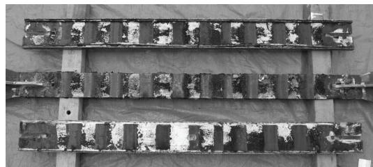
**Figure 6.** Failure modes of the core plate, restraining parts and unbonded material (L450)
