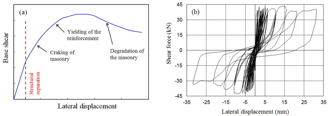
**Figure 3.** Structural response of a confined masonry wall under in-plane lateral loading, (a) typical monotonic response and (b) experimental response (Crisafulli et al. 2005).
