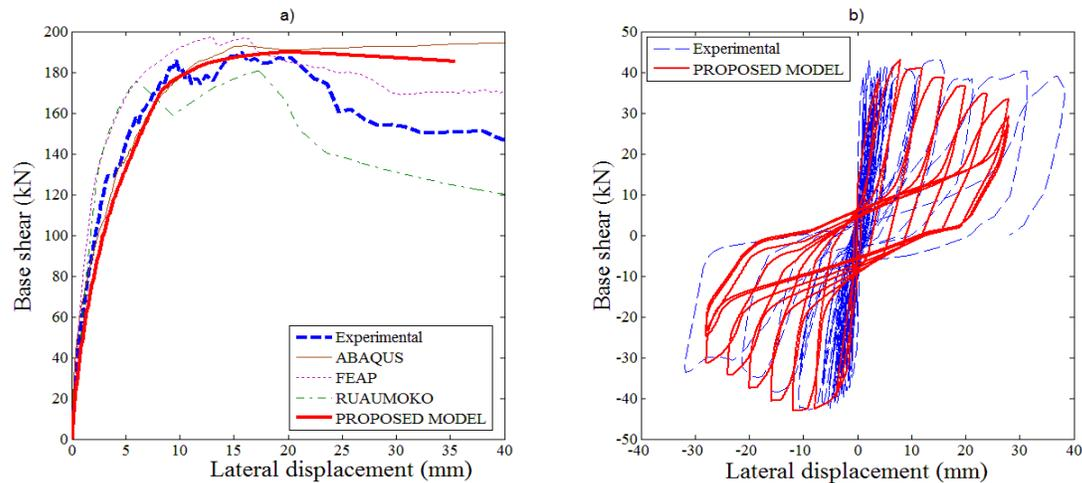
**Figure 10.** Comparison between experimental data and computed results: (a) infilled frame tested by Mehrabi et.al., 1996, and (b) confined masonry wall tested by Crisafulli, 1997.
