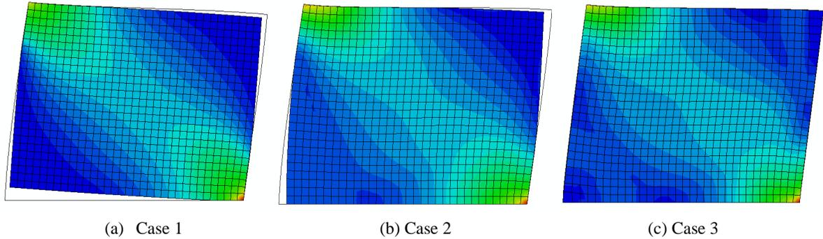
**Figure 5.** Compressive principal stresses in the masonry panel at a force level of 90 kN.
