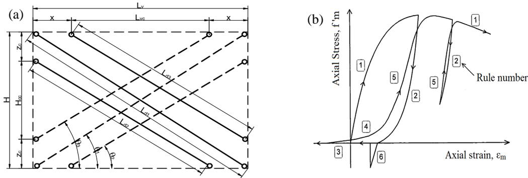
**Figure 8.** Proposed panel macro-element, (a) geometric and mechanical configuration and (b) hysteretic rule for struts the masonry.
