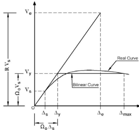
**Figure 4-16.** Generic base shear versus roof displacement envelope curves
