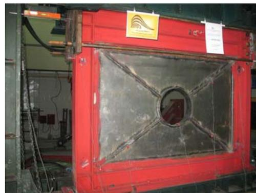
**Figure 5.** Special perforated specimen, SPSW(s4)
