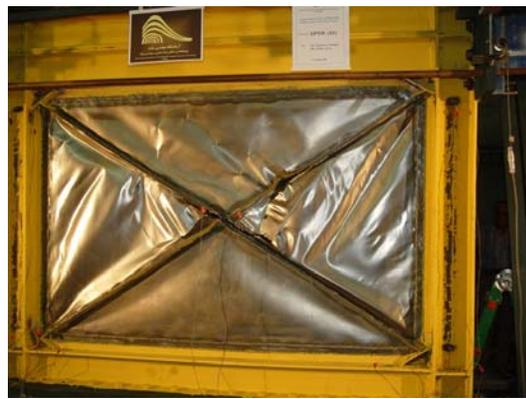
Figure 7. SPSW(s1) at 4.7% drift, in cycle 28
