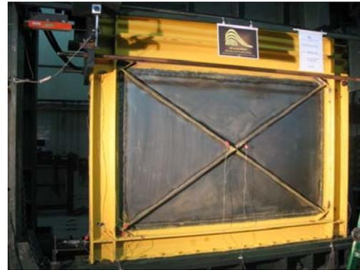
**Figure 3.** Diagonally stiffened specimen, SPSW(s1)
