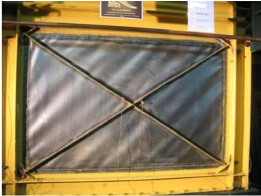
Figure 6. SPSW(s1) at 0.86% drift, in cycle 13
