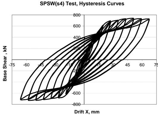
Figure 14. Envelope curves of SPSW(s4)
