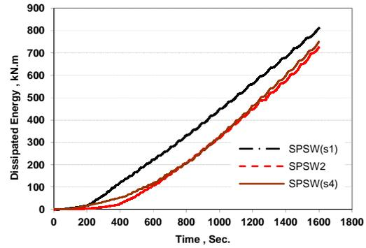
Figure 15. Cumulative Dissipated Energies by the specimens in the cyclic tests
