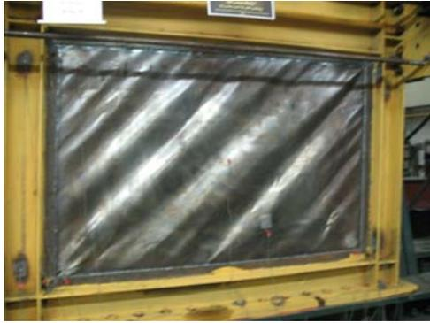
**Figure 8.** SPSW2 at 2.5% drift
