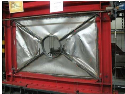
**Figure 11.** SPSW(s4) at 4.4% drift, in cycle 28
