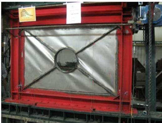
**Figure 10.** SPSW(s4) at 0.56% drift, in cycle 13
