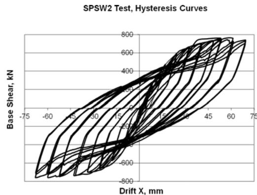
Figure 13. Envelope curves of SPSW2
