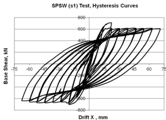
Figure 12. Envelope curves of SPSW(s1)
