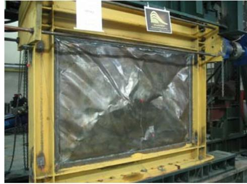
**Figure 9.** SPSW2 at 4.56% drift, in cycle 28
