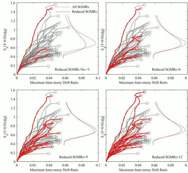
Figure 8. The effect of number of selected SGMRs on the probability density function of collapse capacity using the improved fitness function for the 3-storey RC structure.
