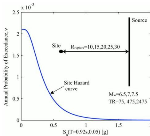
Figure 2 Different parameters used in sensitivity analysis and sample hazard curve for  $T=0.92$ sec,  $M=7$  and  $TR=475$
