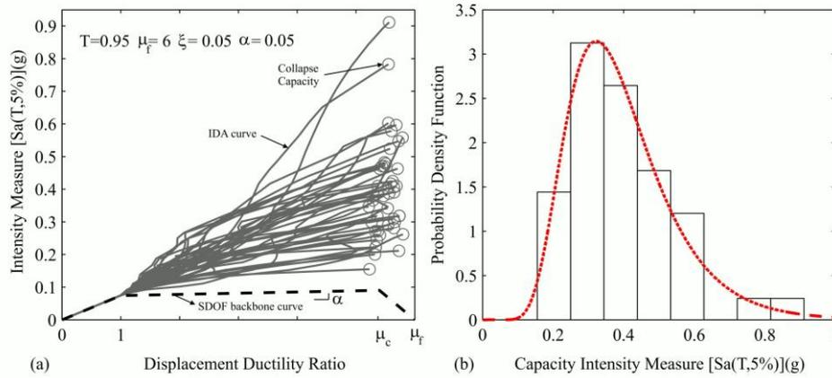
Figure 3. (a) IDA curves for a sample SDOF system with  $T=0.95$ sec,  $\mu=6$ ,  $\xi=0.05$ ,  $\alpha=0.05$  and (b) The distribution of collapse capacity.
