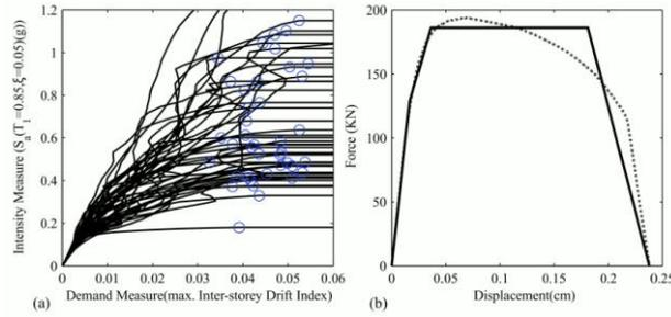
Figure 7. (a) IDA curves; (b) pushover curve in X direction and the equivalent idealized SDOF behaviour.
