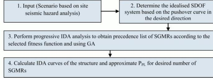
Figure 6 Steps involved in determination of  $P_{PL}$  using progressive IDA
