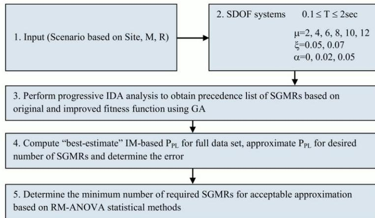
Figure 1. Process of the improved progressive IDA for the purpose of  $P_{PL}$  computation.
