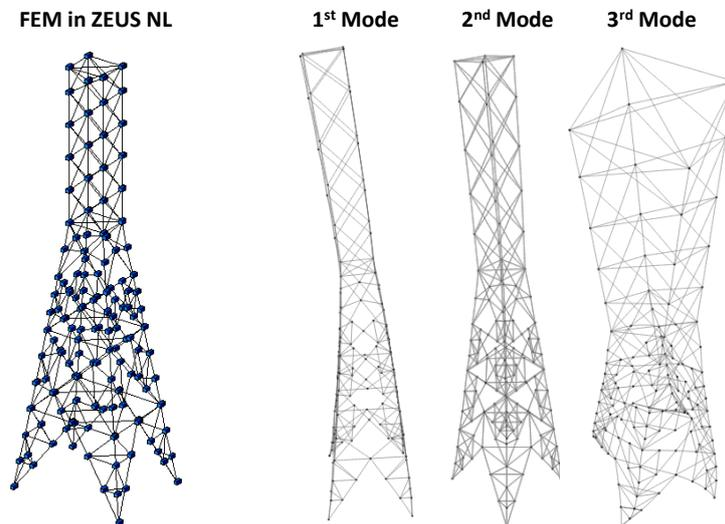
**Figure 3.1.** Finite element model (FEM) in ZEUS NL (Elnashai et al., 2010), and first three mode shapes
