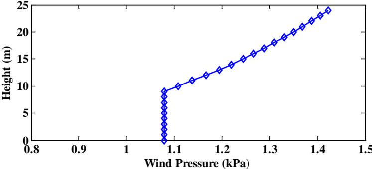
**Figure 2.2.** Wind pressure acting on the tower as a function of height
