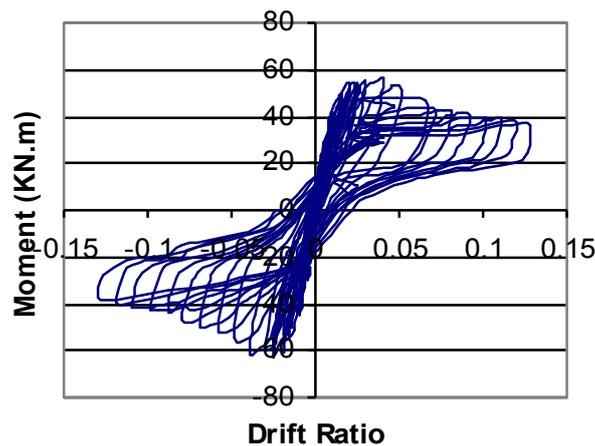
**Figure 14.** The hysteretic behaviour of the column specimen CS-S32-A
