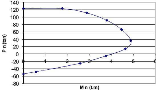
Figure 2. the force-moment interaction diagram of the studied columns
