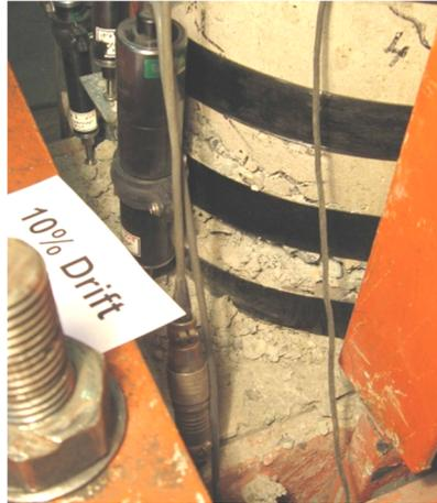
**Figure 11.** The state of damage to the column specimen CS-S64-P at 10% drift ratio
