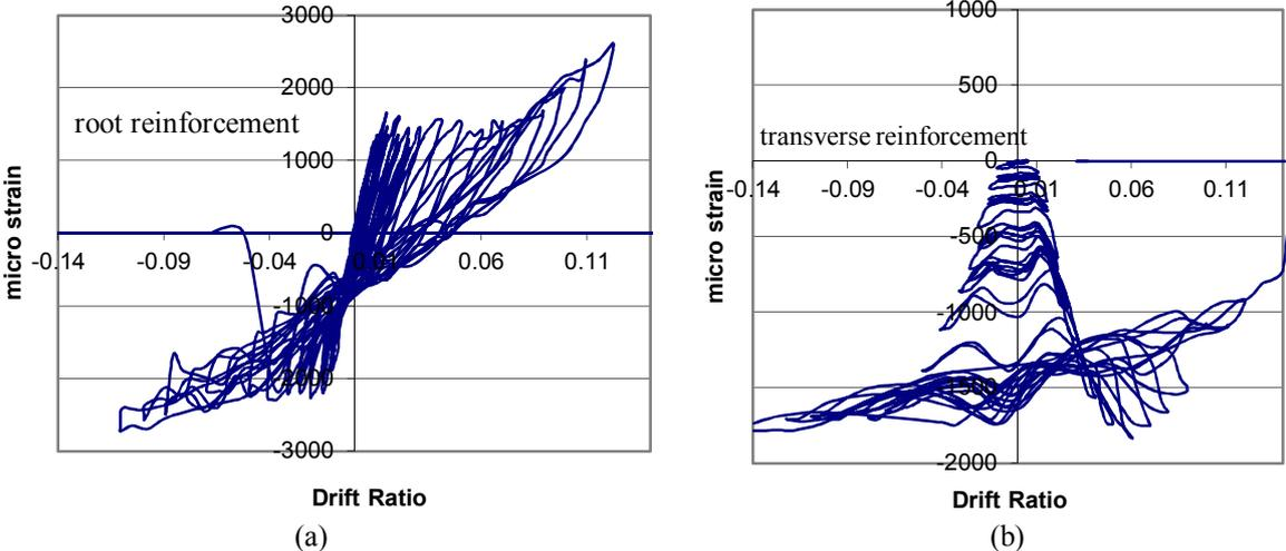
**Figure10.** Variations of the strain on reinforcements of the column specimen CS-S64-A a) On root rebar
