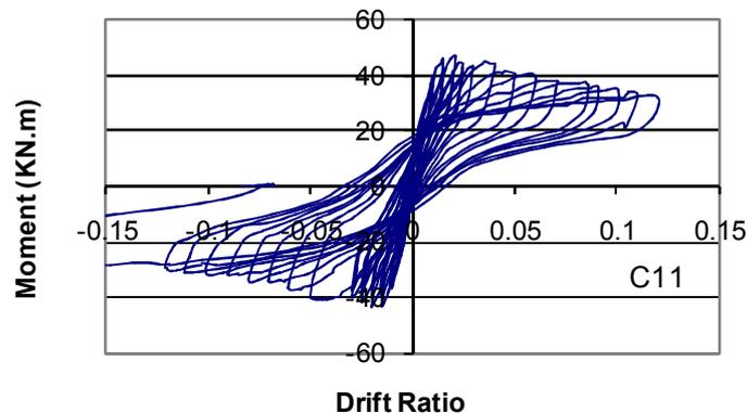
**Figure 12.** The moment-drift ratio capacity curve of the column specimen CS-S64-P
