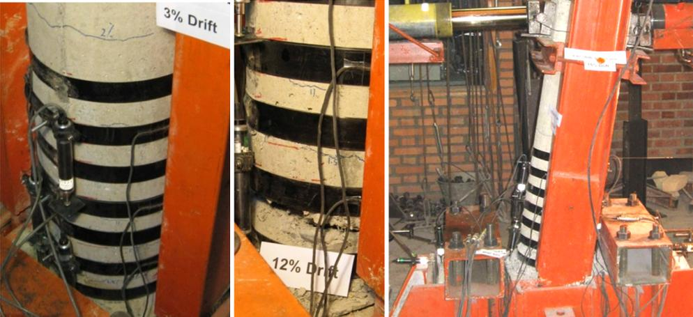
Figure 8. The observed behaviour of the column specimen CS-S64-A at various levels of lateral displacement
