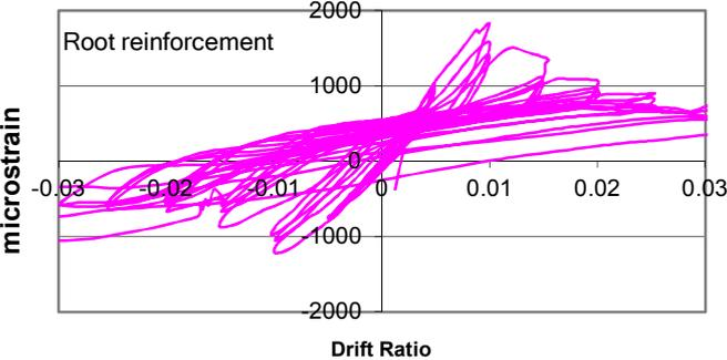
Figure7. Variations of the strain on root rebar of the column specimen CS0
