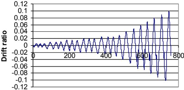
Figure 5. The applied displacement protocol
