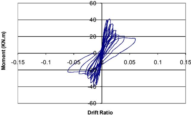
Figure6. The measured moment vs. drift ratio of the column specimenCS0
