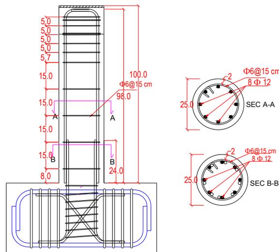
**Figure 1.** Geometry and details of reinforcements of the tested column specimens
