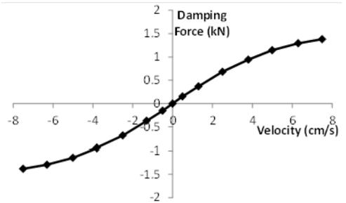
Fig.8 Performance of damper at calculated natural frequency of the structure, 0.8Hz
