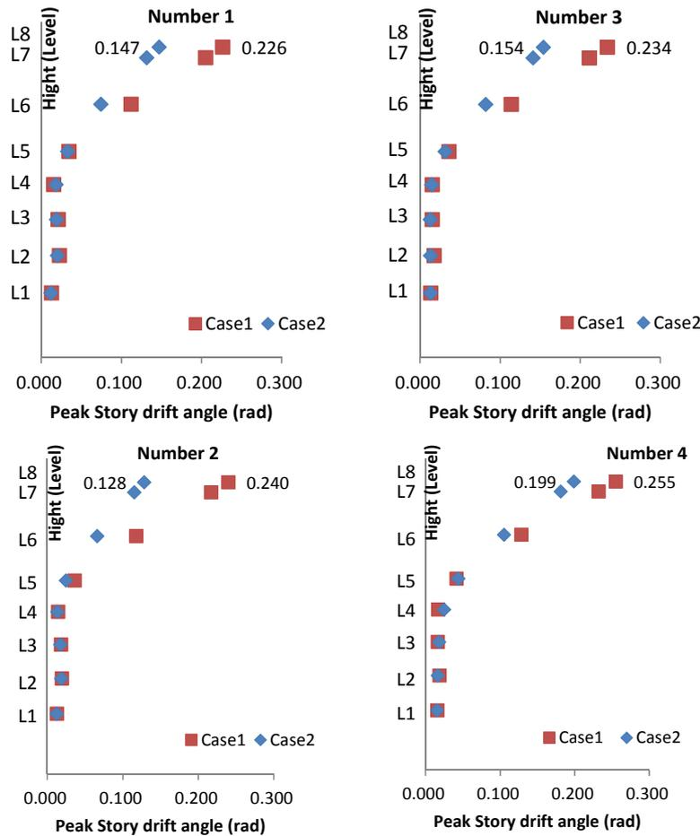
Fig.13 Peak drift angle of central mast ; comparison of the response with and without vibration control device
