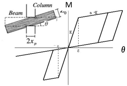
Fig.6 semi-rigidity model of joint of penetrating beam and column
