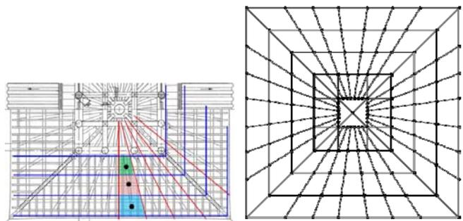
Fig.10 distribution of mass at roof frame
