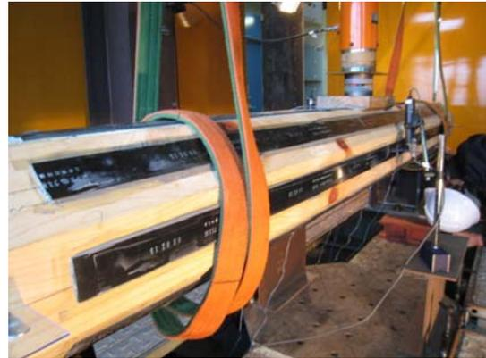
Photo.1 Static flexural test of the central mast model strengthened by carbon fiber bands
