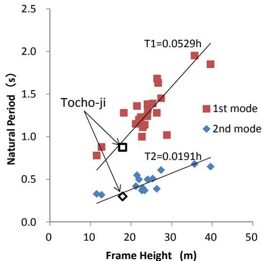
Fig.14 Relationship between frame height and natural period by microtremore measurements
