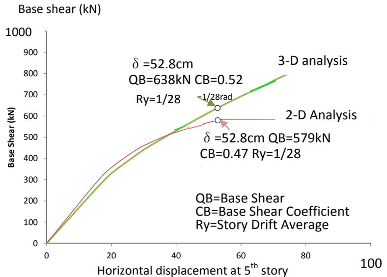
Fig.12 Relationship between base shear and horizontal displacement at 5<sup>th</sup> story ; ultimate lateral strength
