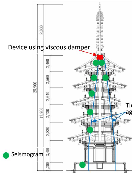
Fig.2 Elevational section of the pagoda with device, wind strengthening and seismograms
