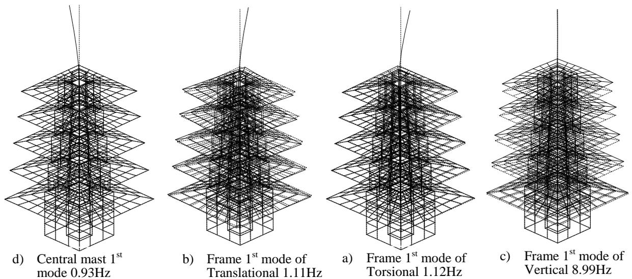
Fig.11 Vibration modes of 3-dimensional model (See Table 2)
