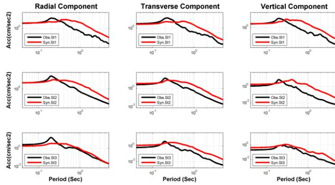
**Fig. 13** Observed (black) and synthetic (red) response spectra (5% damping) for stations 1-3.
