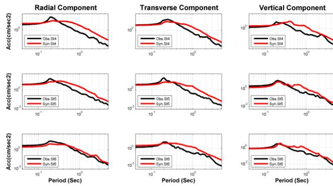
**Fig. 14** Observed (black) and synthetic (red) response spectra (5% damping) for stations 4-6.
