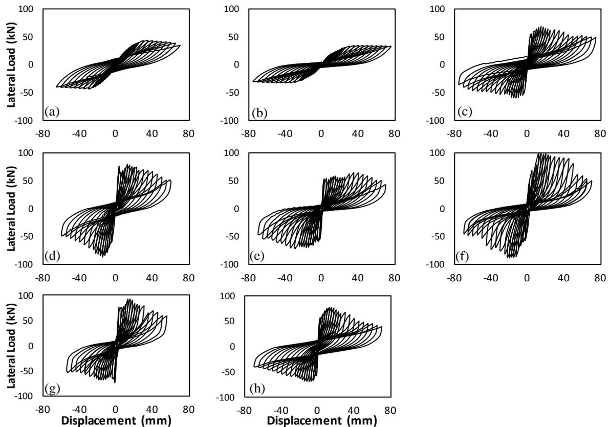
**Figure 3.** Hysteretic behavior of infilled frames; (a) ductile bare frame, (b) non ductile bare frame, (c) ductile frame infilled with full scale bricks; (d) non ductile frame infilled with full scale bricks; (e) ductile repaired frame infilled with full scale bricks; (f) non ductile repaired frame infilled with full scale bricks; (g) ductile frame infilled with half scale bricks; (h) non ductile frame infilled with half scale bricks.
