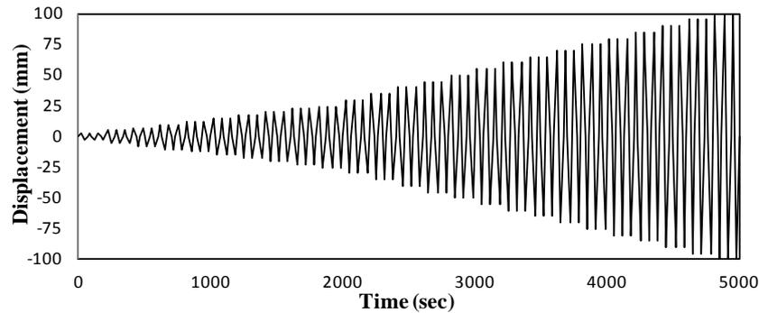
**Figure 2.** Displacement history applied on specimens.
