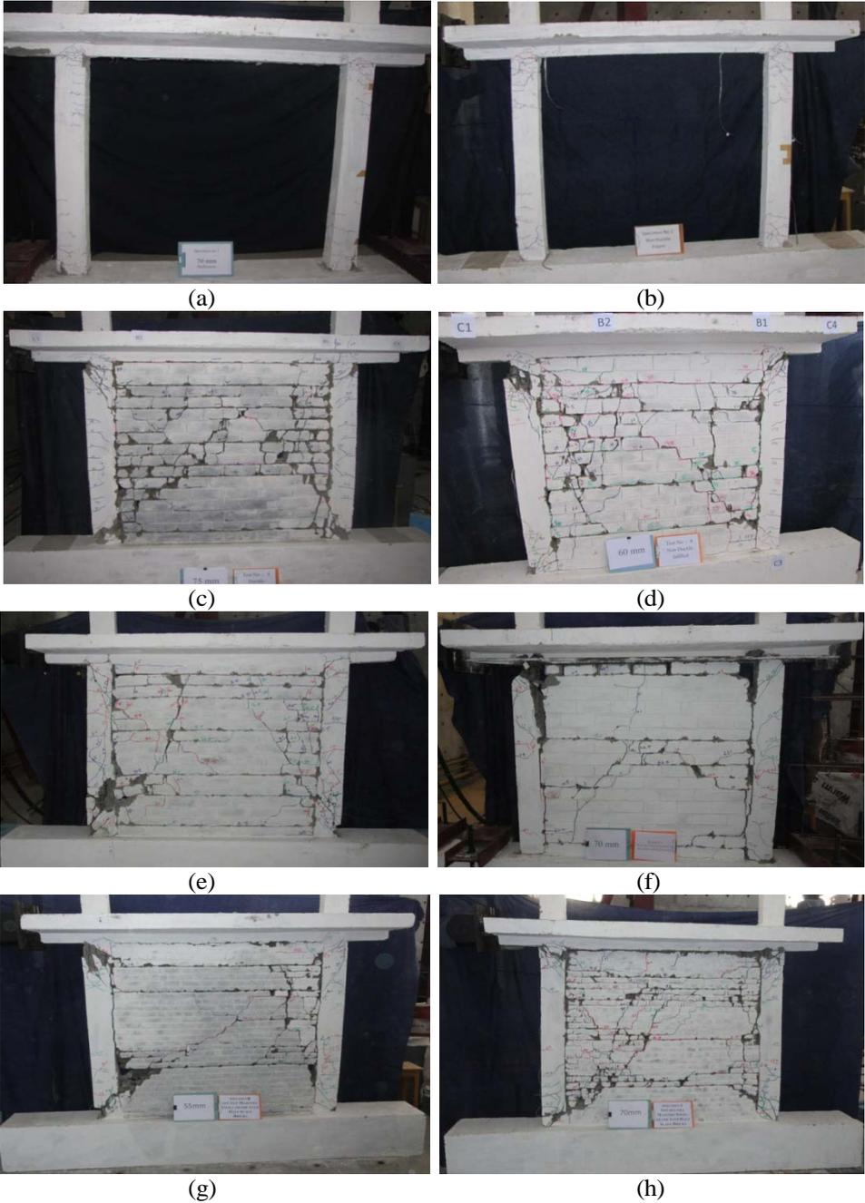
**Figure 4.** Failure mechanisms of infilled frames; (a) ductile bare frame, (b) non ductile bare frame, (c) ductile frame infilled with full scale bricks; (d) non ductile frame infilled with full scale bricks; (e) ductile repaired frame infilled with full scale bricks; (f) non ductile repaired frame infilled with full scale bricks; (g) ductile frame infilled with half scale bricks; (h) non ductile frame infilled with half scale bricks.
