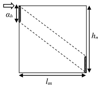
**Figure 5.** Estimation of actual shear demand on RC columns of masonry infilled RC frames
