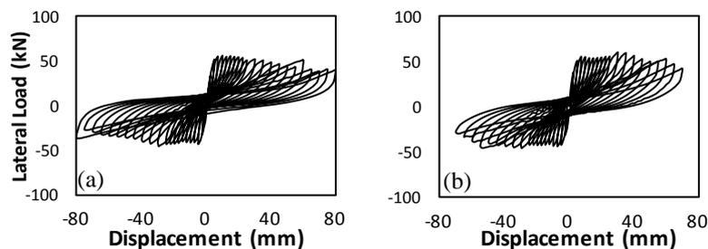
**Figure 6.** Hysteretic behavior of infilled frames: (a) ductile frame infilled with full scale bricks with improved shear capacity throughout the column length; (b) ductile frame infilled with full scale bricks with improved shear capacity in critical regions.
