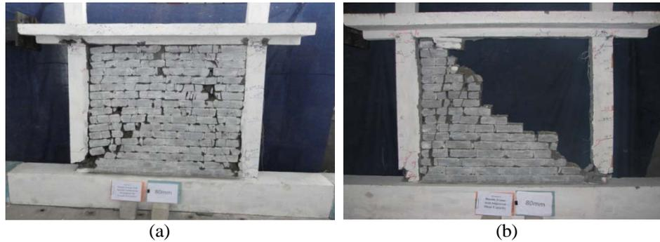
**Figure 7.** Failure modes: (a) ductile infilled frame with full scale bricks with improved shear capacity throughout the length of the column; (b) ductile infilled frame with full scale bricks with improved shear capacity in critical regions.
