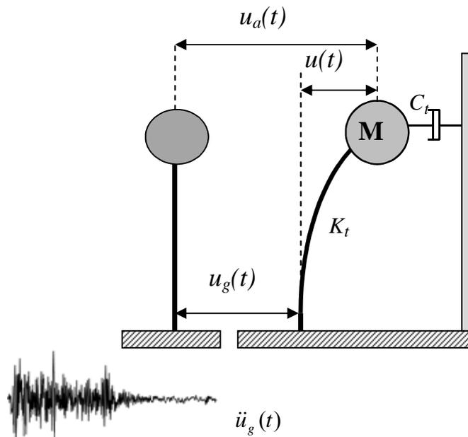
**Figure 2.1.** Bridge with a single degree of freedom.
