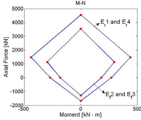
**Figure 2.** Axial force - bending moment interaction
