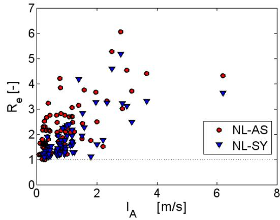
**Figure 6.** Reduction factor versus Intensity arias
