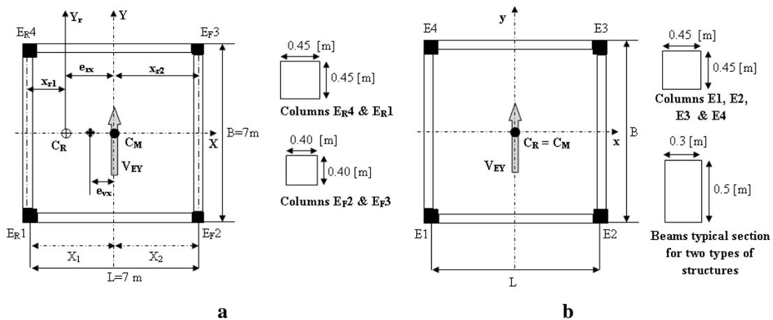
Figure 1. Geometry and transverse section description of structures
