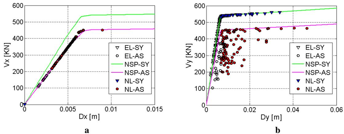
**Figure 3.** Base shears versus Top displacements in both directions X and Y
