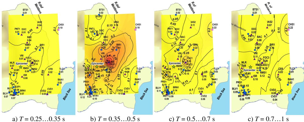
**Figure 3.2.** Damage maps for the August 30, 1986 earthquake.  $C_y=0.30$ , maximum monotonic ductility  $\mu_{mon}=6$
