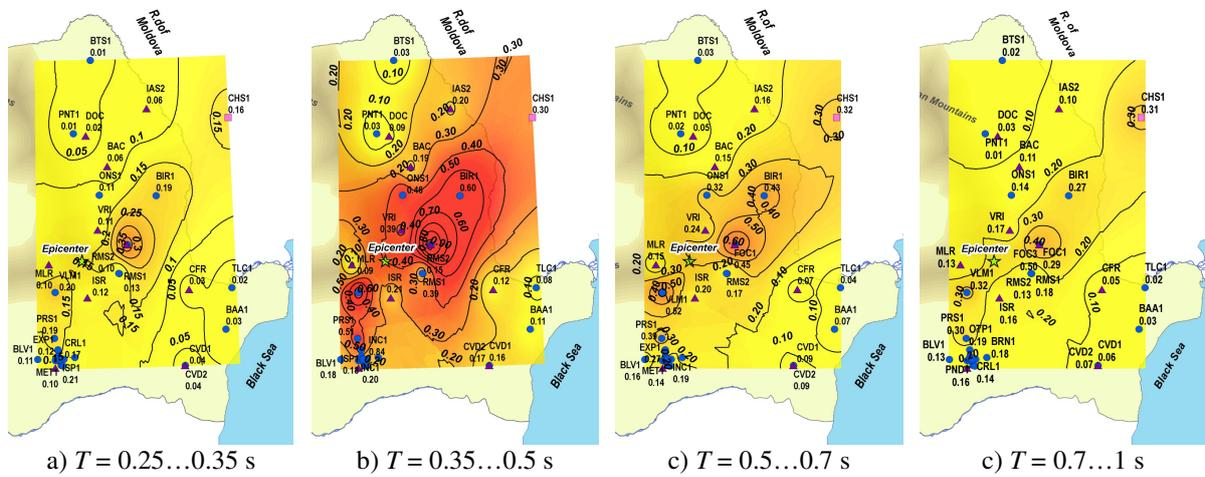
**Figure 3.1.** Damage maps for the August 30, 1986 earthquake. Yield strength coefficient  $C_y=0.20$ , maximum monotonic ductility  $\mu_{mon}=6$
