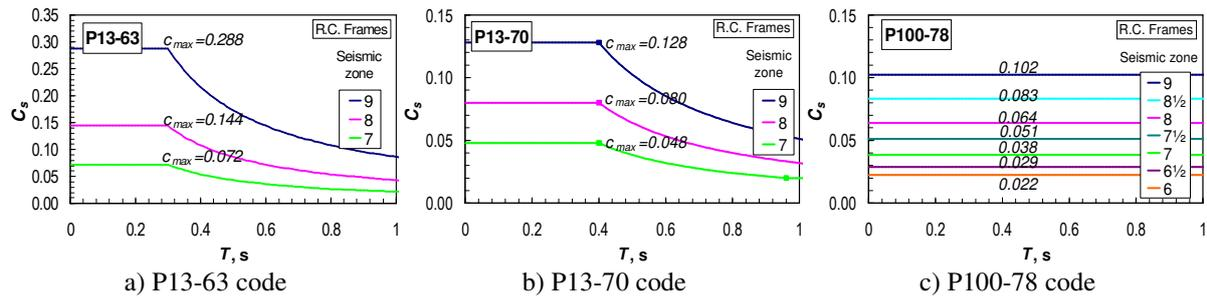
**Figure 4.1.** Base shear coefficients,  $C_s$ , for reinforced concrete frames, according to three consecutive Romanian seismic codes
