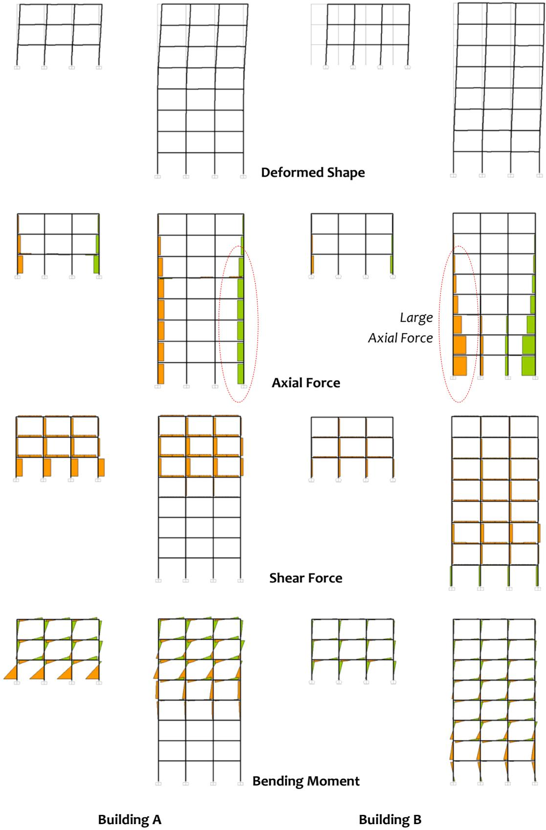
**Figure 3.4** Deformed Shape, Axial Force, Shear Force and Bending Moment Diagram for Building A and Building B subjected to lateral load; the frames shown are along ROAD direction
