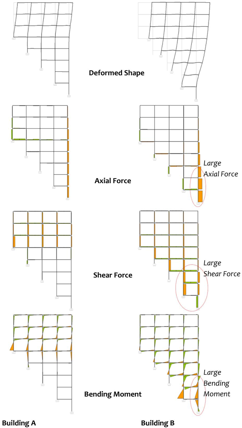
**Figure 3.3** Deformed Shape, Axial Force, Shear Force and Bending Moment Diagram for Building A and Building B subjected to lateral load; the frames shown are along VALLEY direction
