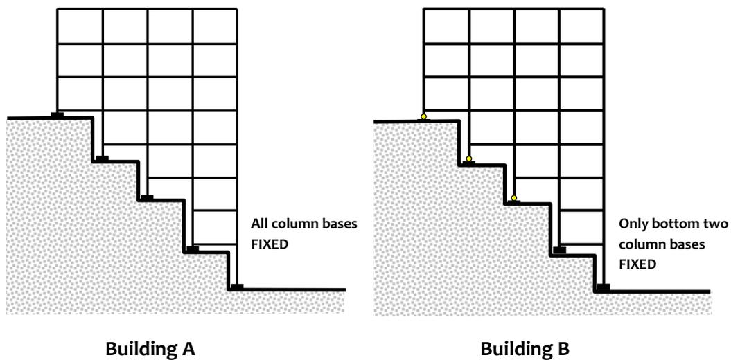
Figure 3.2 Building with different support conditions
