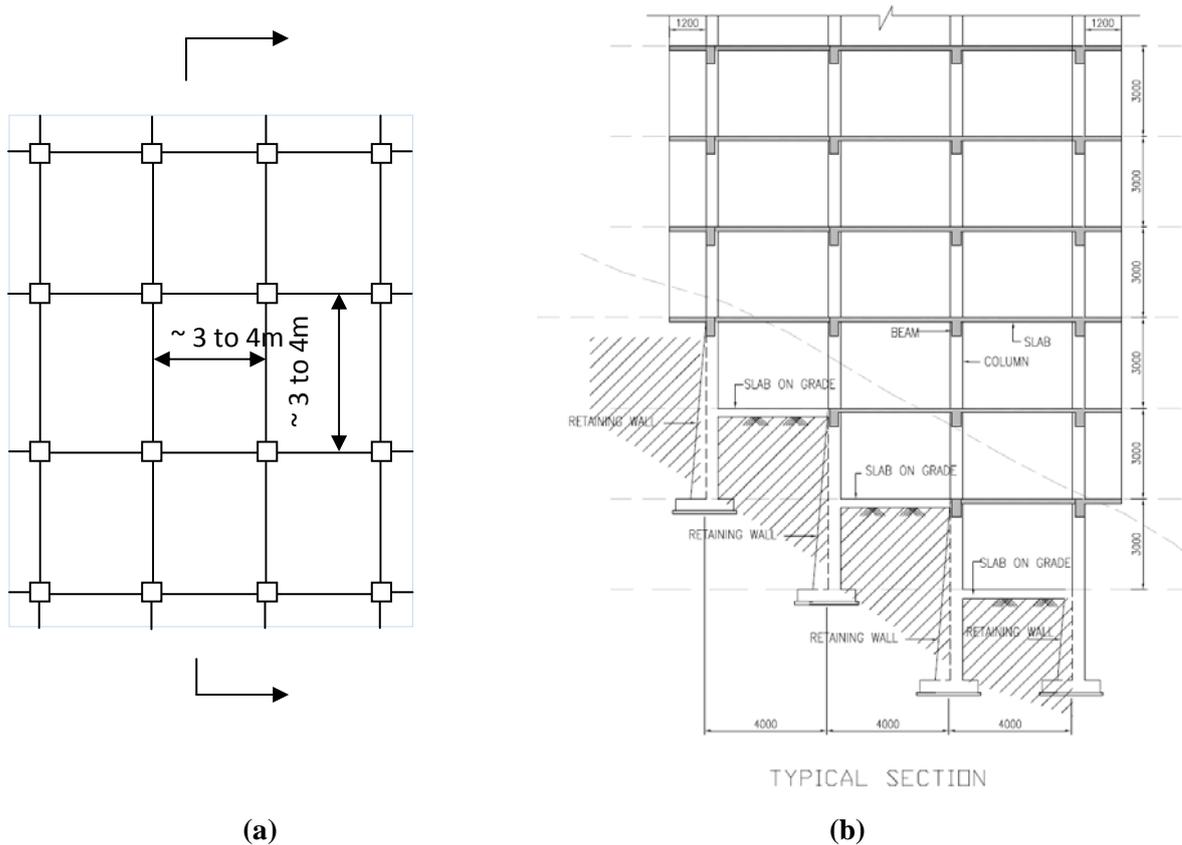
**Figure 3.1** Typical RC frame building along hill slopes (a) building plan, and (b) and sectional elevation [Courtesy: Alpa Sheth, Mumbai]
