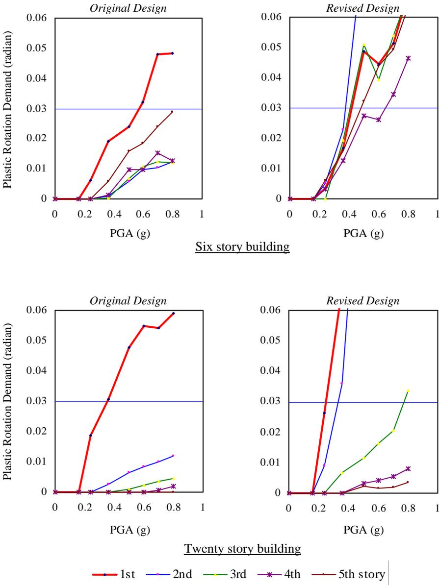
**Figure 3.4.** Average plastic rotation demand on connections at first five stories under Parkfield motion with PGA scaled to 0.36g
