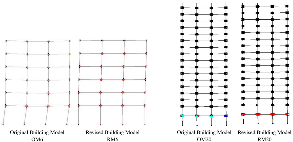
**Figure 3.2.** Plastic hinges at beam and column ends under Parkfield motion with PGA scaled to 0.36g
