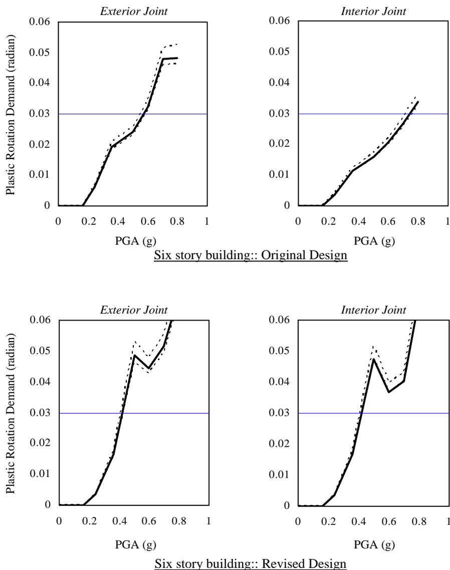
**Figure 3.3.** Plastic rotation demand on connections at first story under Parkfield motion with PGA scaled to 0.36g
