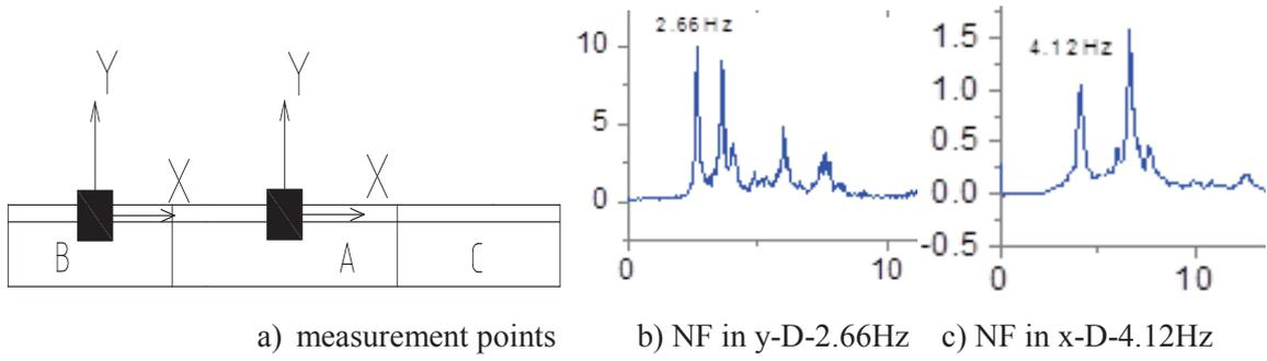
Figure 2. Natural frequency test for the seismic damaged LCBCM school building
