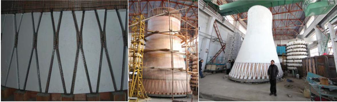
Figure 3. Construction of the 1:30 model cooling tower structure to be tested on shaking table
