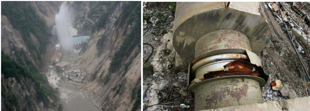
**Figure 7.** Failure of penstock near Shapai powerhouse: Water jet from failed expansion joint and flooding of powerhouse area (left) and detail of damaged expansion joint (right) (Wenchuan earthquake, China)
