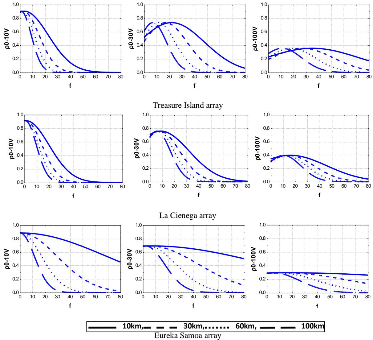
Figure 4.2. Coherency in vertical direction at different epicenter distances
