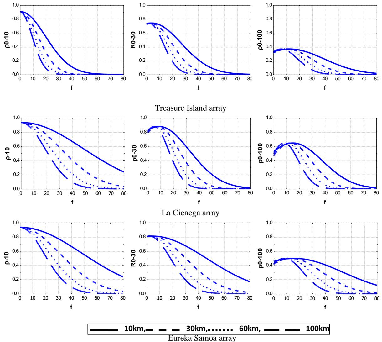
**Figure 4.1.** Coherency in horizontal direction at different epicenter distances
