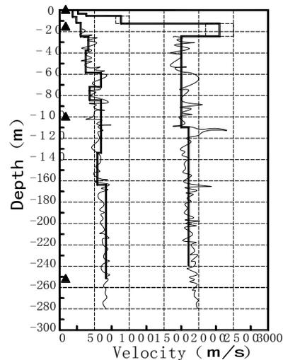
**Figure 2.2.** P and S wave velocity at La Cienega array
