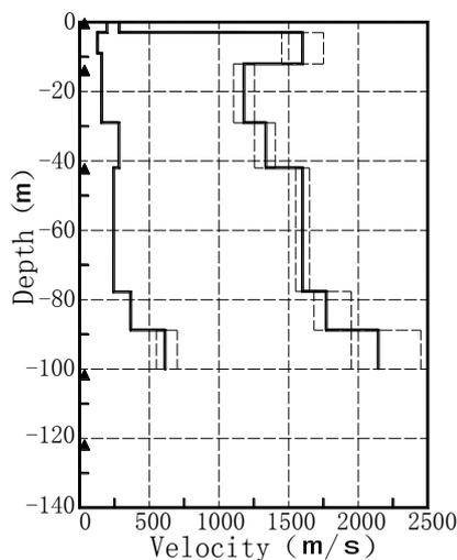
**Figure 2.1.** P and S wave velocity at Treasure Island array
