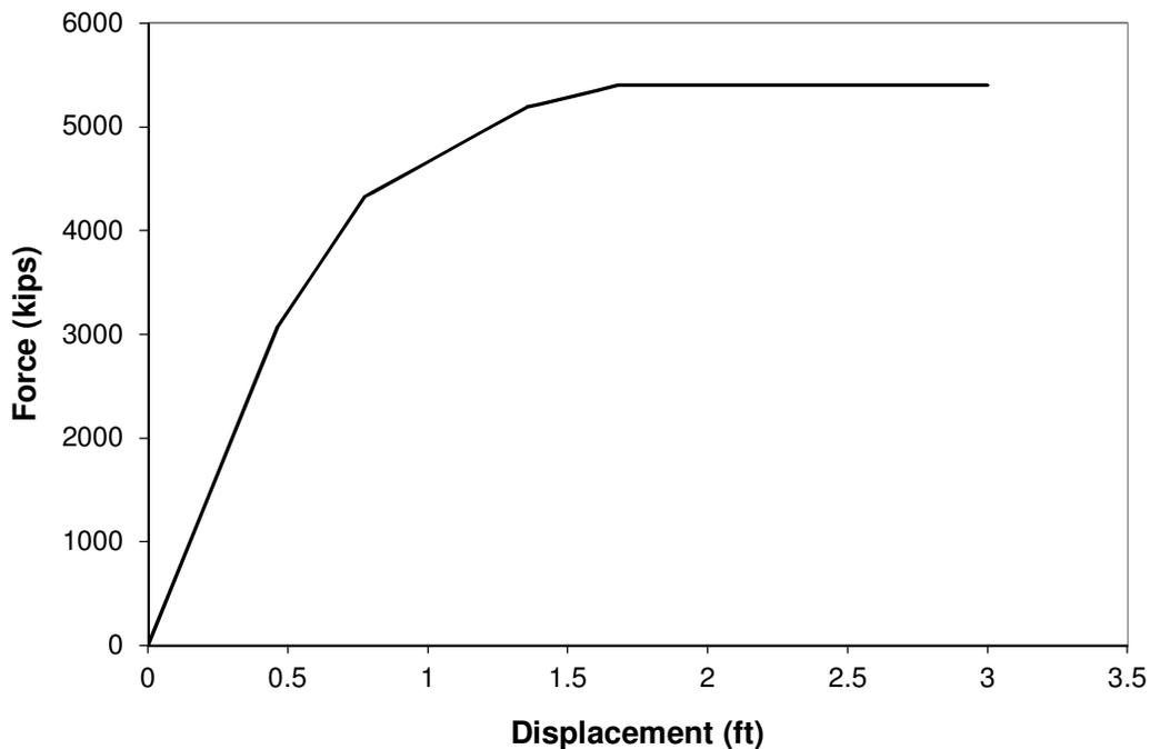
**Figure 3.3.** Monotonic push to 3 ft with all plastic hinges forming
