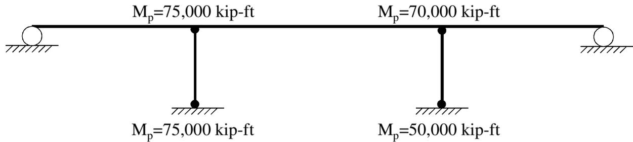
**Figure 3.2.** Plastic moment capacities at the four column plastic hinges
