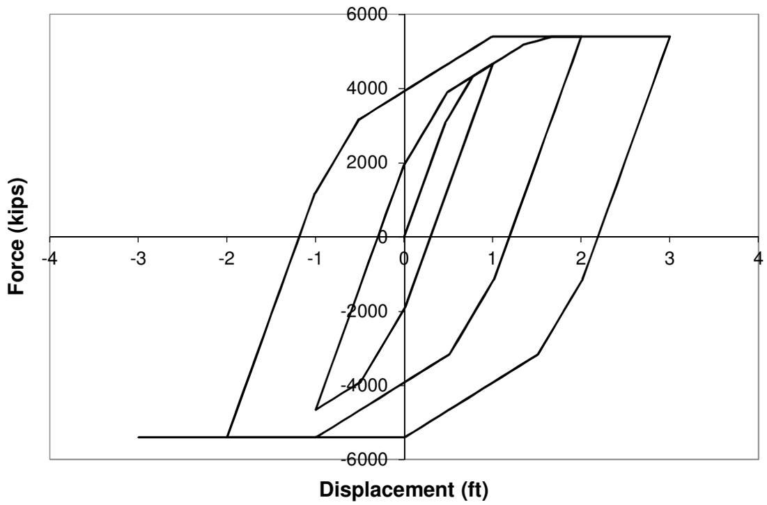
**Figure 4.3.** Frame displacements (in ft) of 1, -1, 2, -2, 3, -3
