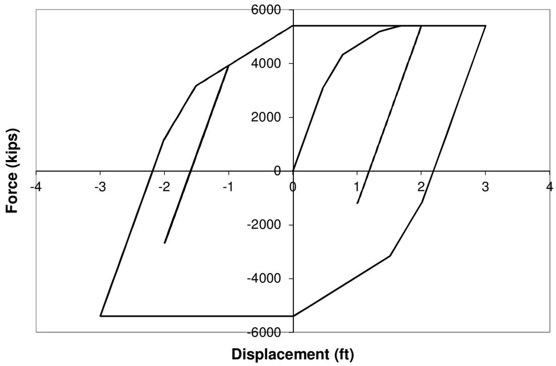
**Figure 4.2.** Frame displacements (in ft) of 3, -3, -1, -2, 2, 1
