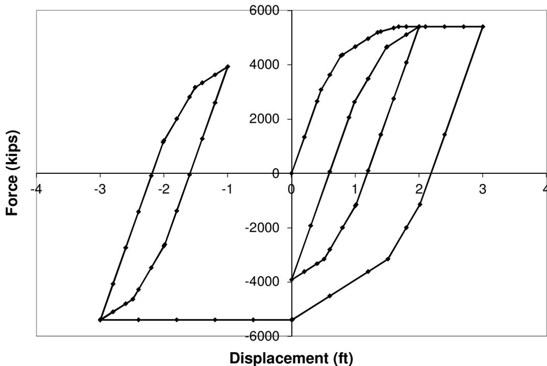
**Figure 4.4.** Frame displacements (in ft) of 2, 0, 3, -3, -1, -3 with each increment indicated
