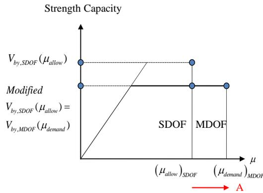
**Figure 3.1.** Comparison of the MDOF ductility demand with the SDOF allowable ductility
