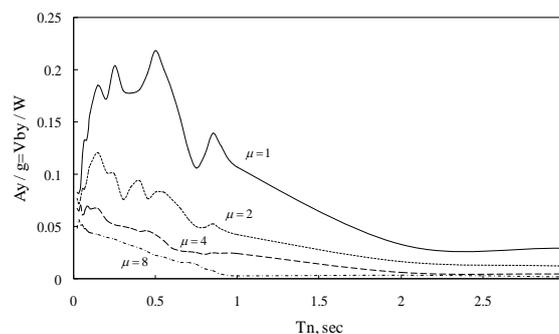
**Figure 3.2.** Constant ductility response spectrum for El Centro ground motion
