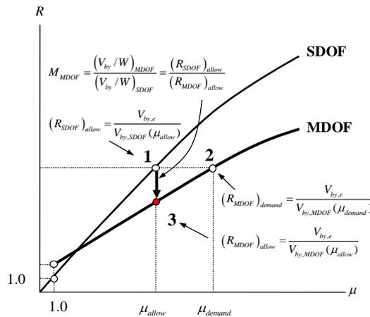
Figure 3.7.  $R$ - $\mu$  relationship between the SDOF and MDOF systems
