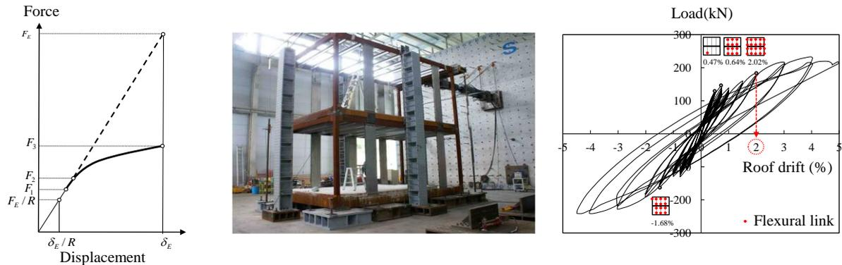
(a) Components of the over-strength factor (b) Test setup and results for a LSP-modular system
