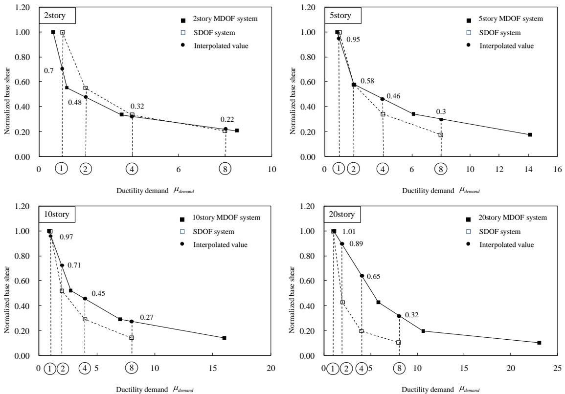
**Figure 3.4.** Relationship between the normalized strength and the ductility demand
