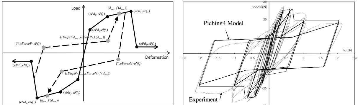
(a) Definition of the Pinching4 material model (b) Comparison of the test results with the pinching4 model
