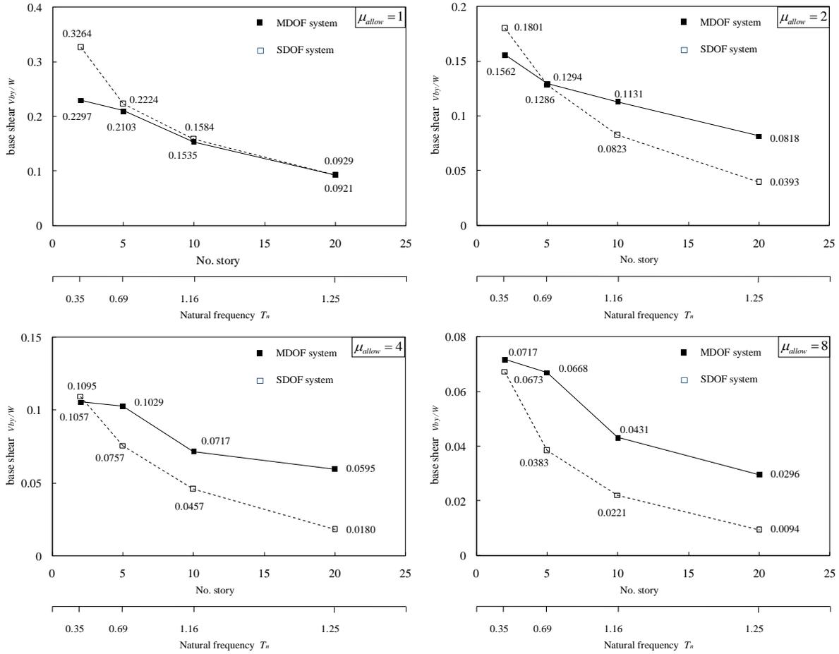
Figure 3.5. Base shears of MDOF and corresponding SDOF systems
