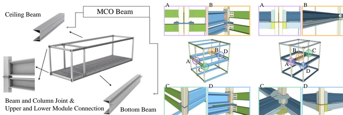
(a) MCO beams (b) End-plate connection (c) Bracket connection
