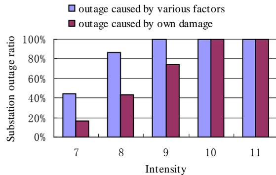
**Figure 4.2.** Distribution map of substation outage ratio in different intensity zones
