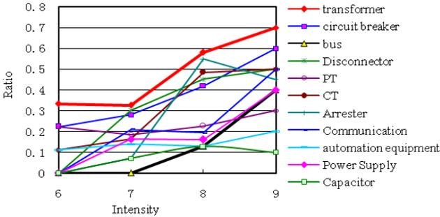
**Figure 4.3.** Damage frequencies of various equipments in damaged substations
