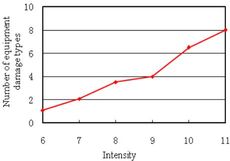
**Figure 4.4.** Relation between intensity and the average number of the Equipment damage type
