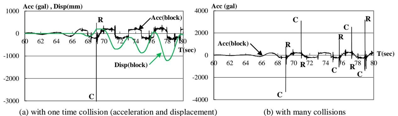
Figure 5. Sliding with collision (time history of acceleration on the block)
