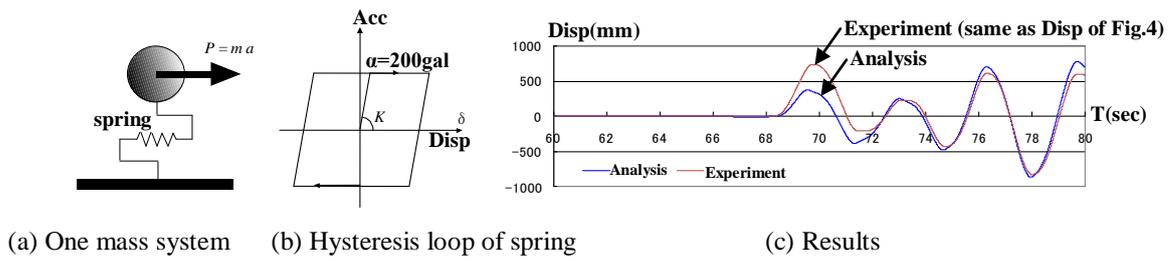
Figure 7. Time history of displacement (experimental and analytical results)
