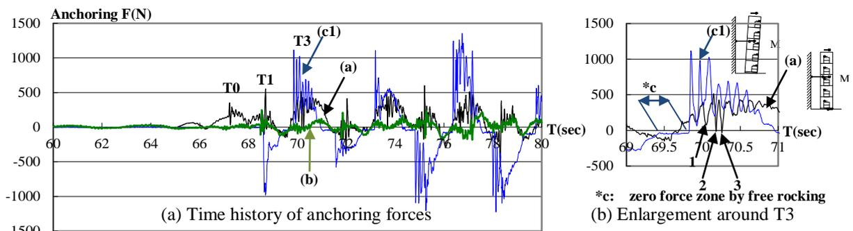
Figure 12. Time history of anchoring forces according to clamp conditions ((a), (b), and (c1))
