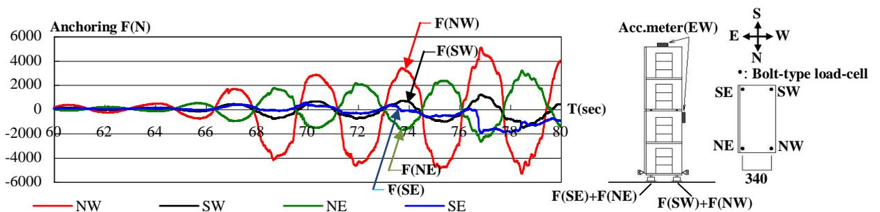
Figure 9. Time history of the anchoring forces in the load cells (SE, NE, SW, and NW)
