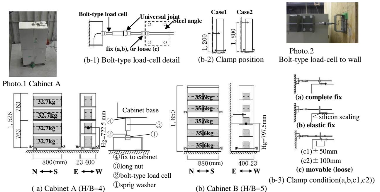
Figure 3. Experimental apparatus for measuring anchoring forces
