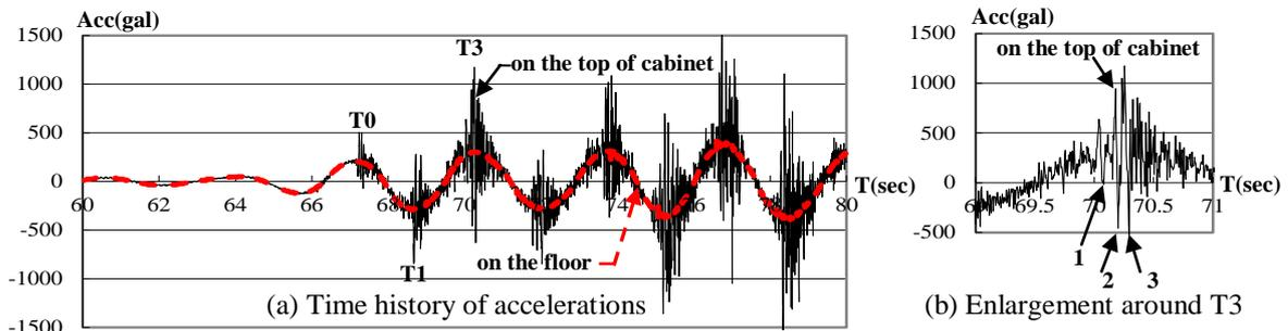
Figure 11. Time history of accelerations (on the floor and on the top of cabinet B)
