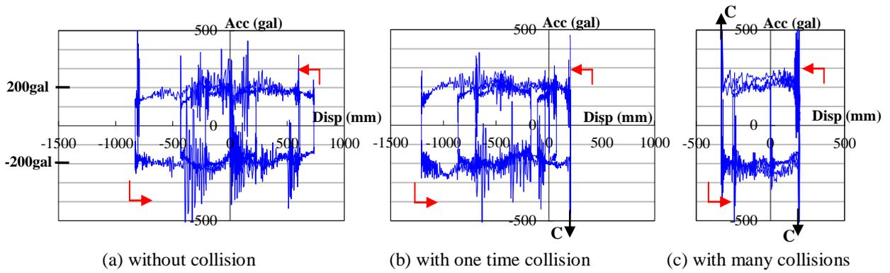
Figure 6. Acceleration and displacement relationship (sliding behaviour)
