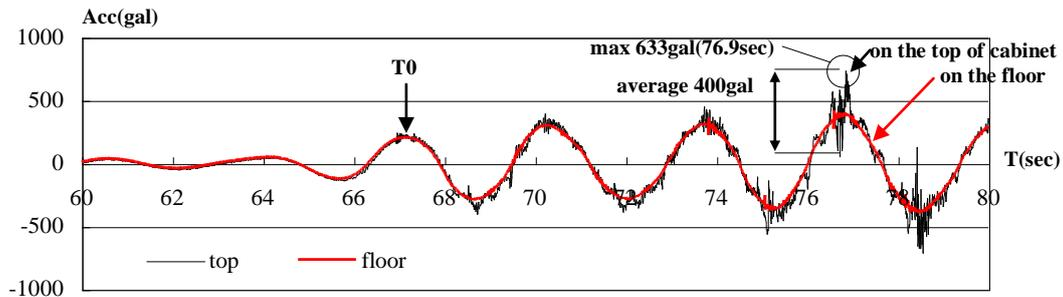
Figure 8. Time history of accelerations (on the floor and on the top of cabinet A)
