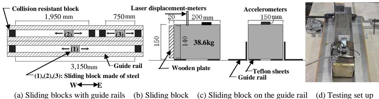
Figure 2. Experimental apparatus for sliding behaviour
