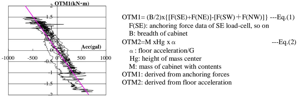
Figure 10. Overturning moment (OTM1 derived from load cell data) and acceleration (cabinet) relationship
