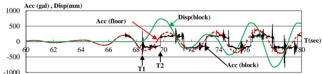
Figure 4. Time history of accelerations (on floor and on block) and relative displacement
