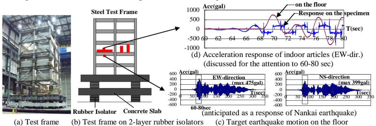
Figure 1. Substructure shaking table test
