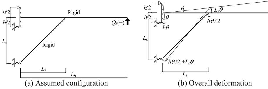
**Figure 4.2** Macro-models for vicinity of beam-column joint and knee brace (the knee brace in tension)
