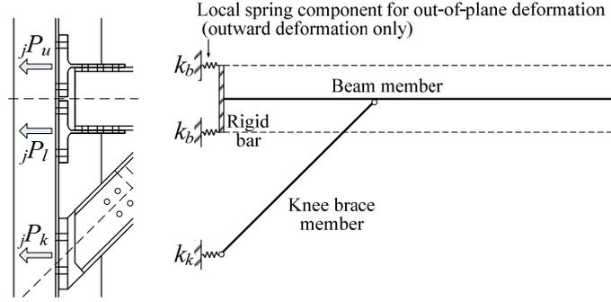
**Figure 4.1** Local out-of-plane spring components at the beam-end and the knee-brace-end
