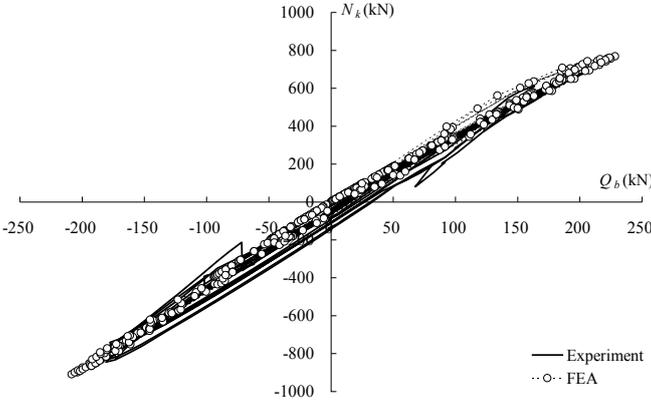
Figure 3.2 Comparison of axial force of knee brace member (T-shaped reinforced specimen)
