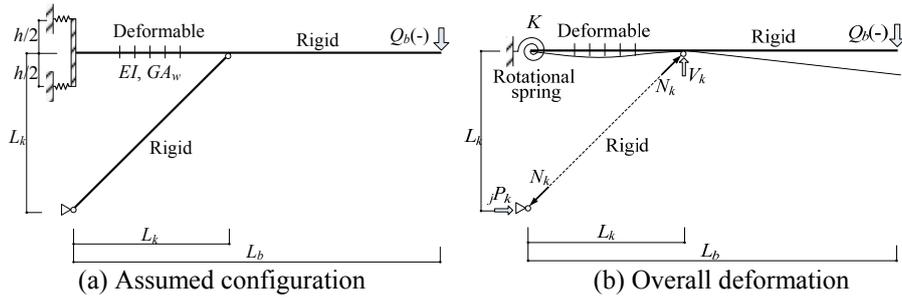
**Figure 4.3** Macro-models for vicinity of beam-column joint and knee brace (the knee brace in compression)
