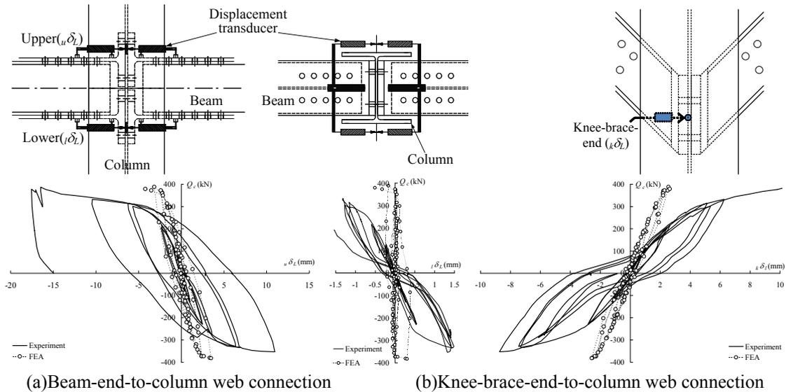
**Figure 3.3** Comparison of out-of-plane deformation of column web plate (cruciform reinforced specimen)
