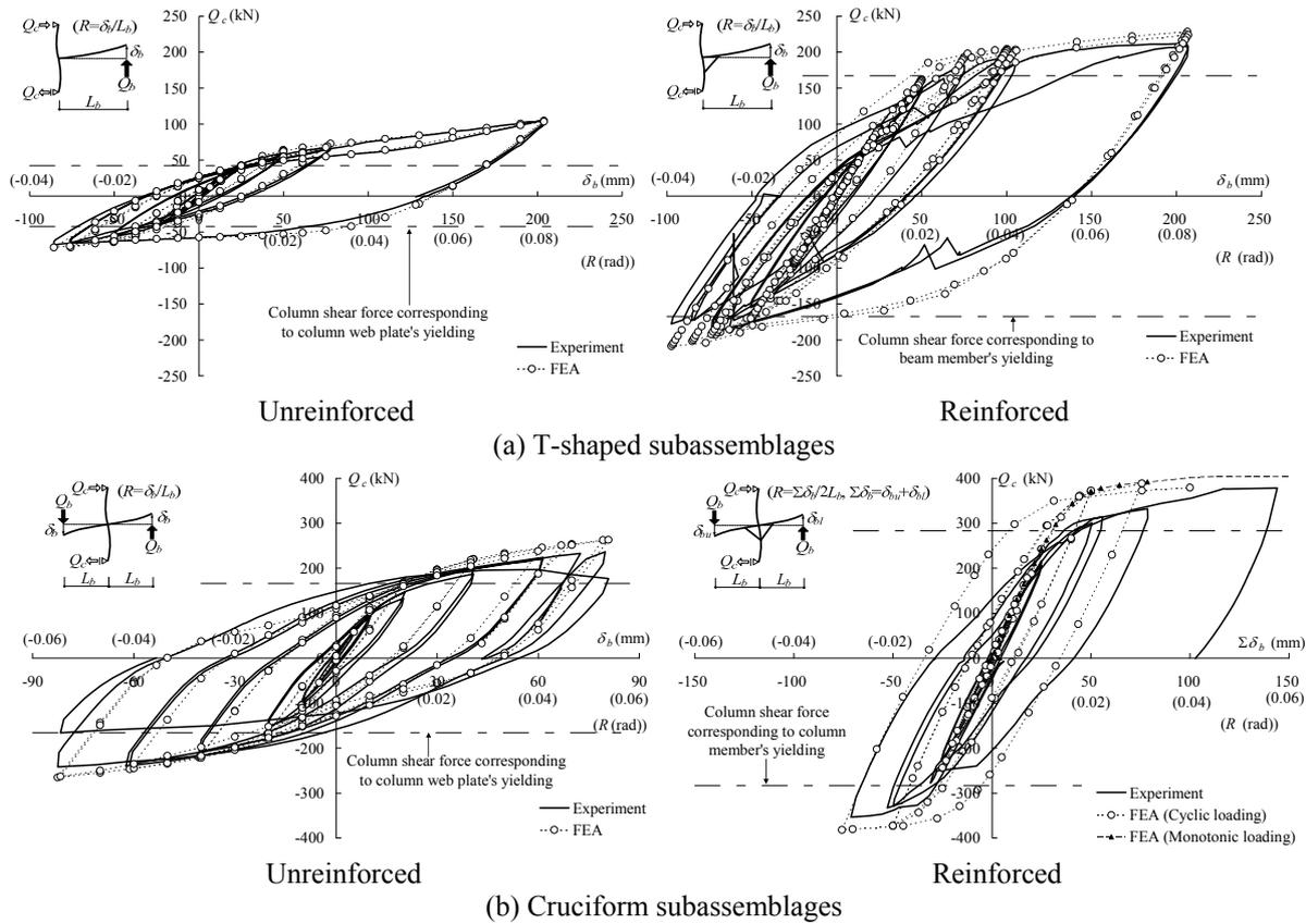
**Figure 2.2** Column shear force ( $Q_c$ )-drift angle ( $R$ ) relationship curves (with FEA results)
