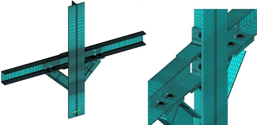
Figure 3.1 Example of finite element model (Cruciform reinforced specimen)
