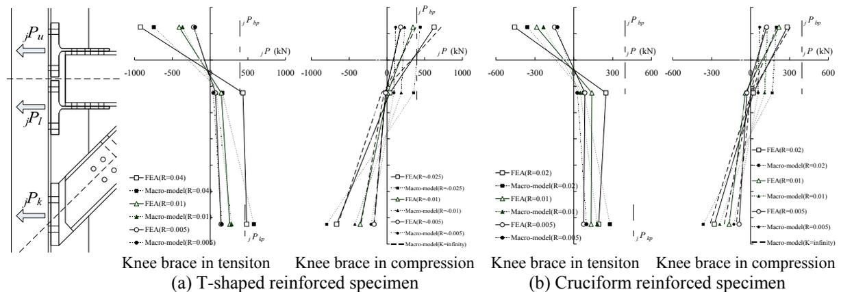
**Figure 4.4** Reaction force distribution at beam- and knee-brace-end bolted joints
