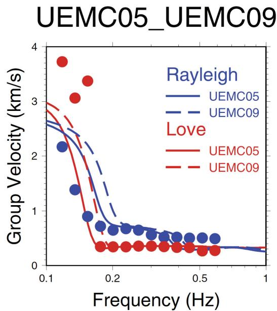
**Figure 4.2.** Dispersion curve of Rayleigh and Love wave group velocity between UEMC05 and UEMC09
