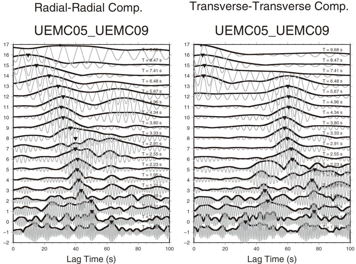
**Figure 4.1.** Envelopes of R-R and T-T components of inter-station Green's function from UEMC05 to UEMC09
