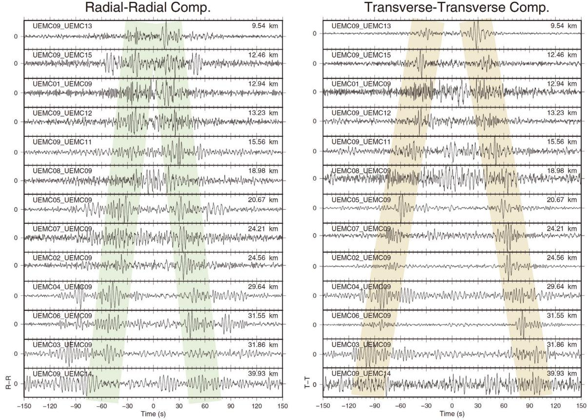
**Figure 3.2.** R-R and T-T components of inter-station Green's functions ordered by the inter-station distance
