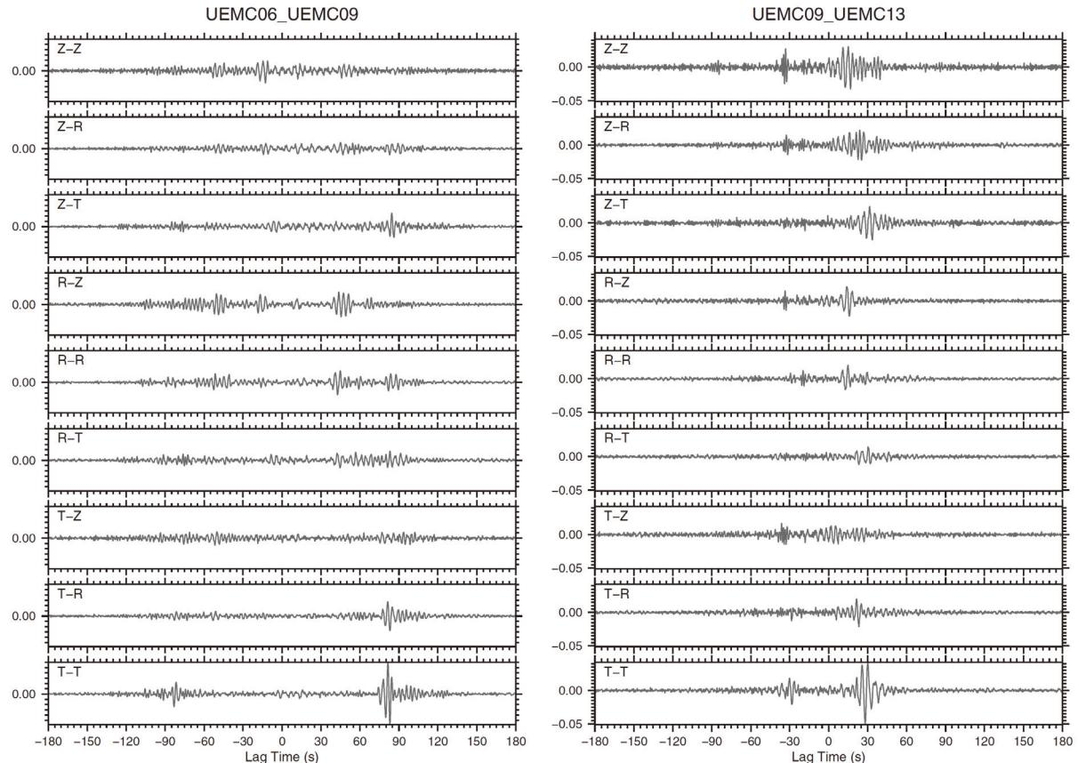
**Figure 3.1.** Example of stacked inter-station cross-correlations (Z: Vertical, R: Radial, T: Transverse comp.)
