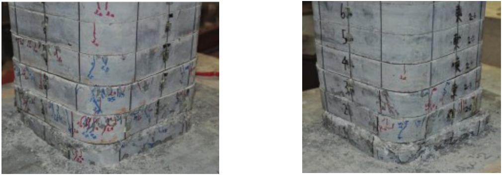
**Figure 6.** The southeast (left) and northwest (right) corners of specimen PC-UFC at drift 3.5%
