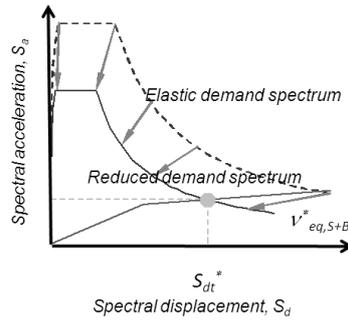
**Figure 5.** Evaluation of the equivalent viscous damping needed to achieve the target performance point
