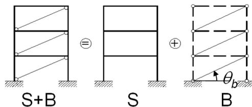
**Figure 1.** Scheme of the braced structure ( $S+B$ ) as sum of the structure ( $S$ ) and the bracing system ( $B$ )
