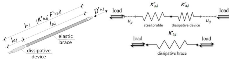
**Figure 6.** Dissipative device “ $j$ ” assembled in series with an extension element (*e.g.* a steel profile): equivalent model of springs in series ( $K'_{d,j}$ ;  $K'_{p,j}$ ) and equivalent single spring model ( $K'_{b,j}$ )
