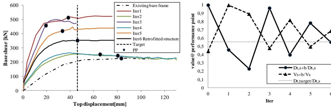
Figure 8. 2D frame: a) BRB effect on capacity curves, b) convergence of the procedure
