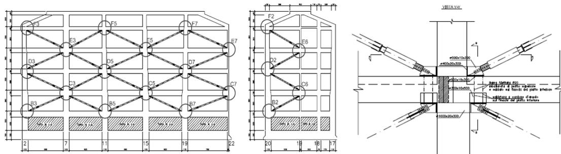
Figure 9. Existing structure: BRB distribution inside the frame (a), detail of BRB connection (b).
