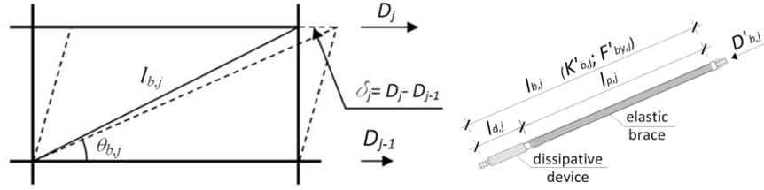
**Figure 3.** Deformed shape of a generic single part of the braced frame
