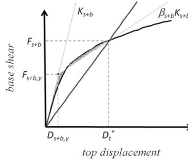
**Figure 4.** Evaluation of the equivalent bilinear capacity curve
