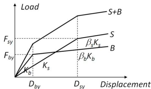
**Figure 2.** Interaction between the structure ( $S$ ) and the bracing system ( $B$ ) expressed in terms of horizontal components of the force-displacement relationship
