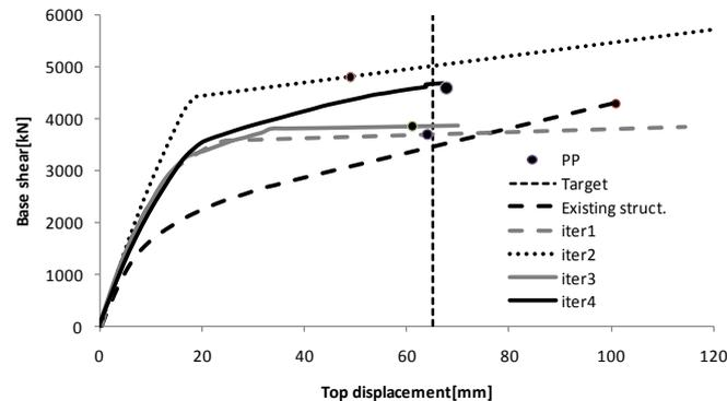
**Figure 10.** Existing structure: capacity curves and performance top displacement at each step.
