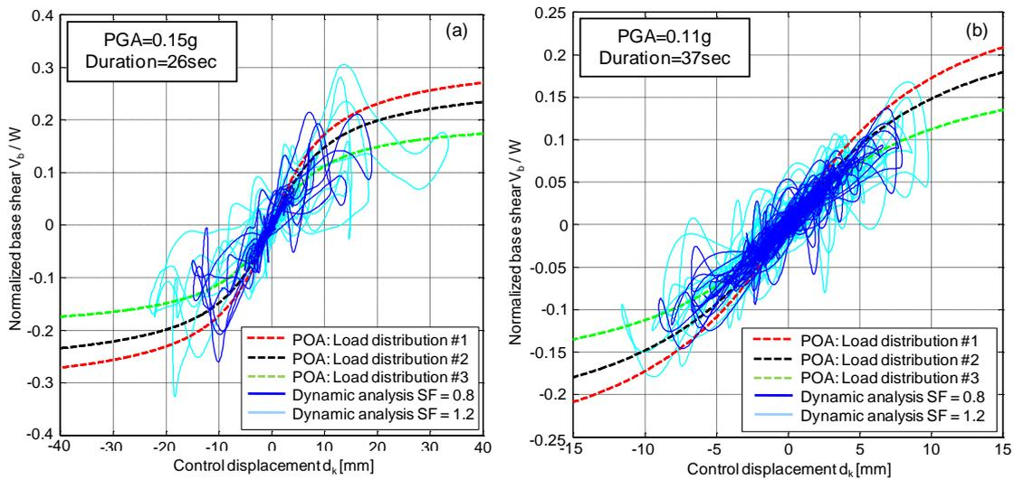
**Figure 3.** Comparison between push-over and non-linear dynamic analyses under two accelerograms from the set: response curves of two dynamic simulations with different scaling factors (SF).
