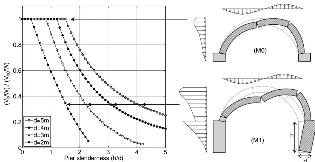
**Figure 5.** Seismic capacity of arches on pillars vs. pillar slenderness for different values of pillar width.
