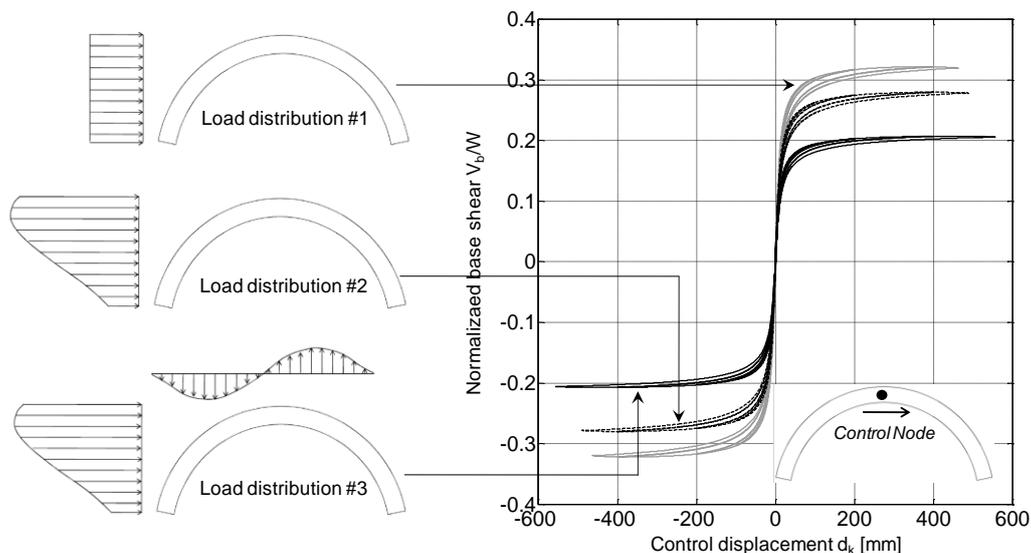
**Figure 2.** Cyclic push-over curves under different load distributions on an arch with  $R=10\text{m}$ ,  $s=0.15R$ ,  $\beta=157.5^\circ$ .
