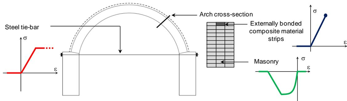
**Figure 6.** Modelling of strengthened arches on pillars.
