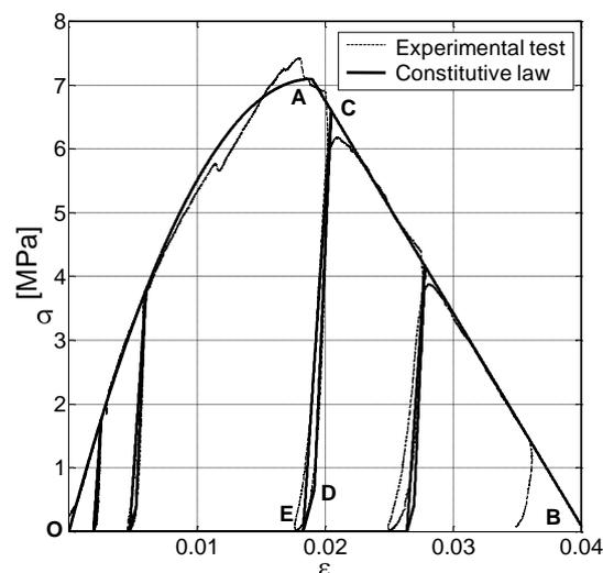
**Figure 1.** Experimental stress-strain curve for a brickwork prism under cyclic compression and uniaxial constitutive relation adopted in numerical simulations (compressive stresses are assumed as positive).
