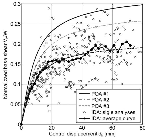
**Figure 4.** Average IDA curve and push-over curves for different load distributions on a circular arch with  $R=10\text{m}$ ,  $s/R=0.15$ ,  $\beta=157.5^\circ$ .
