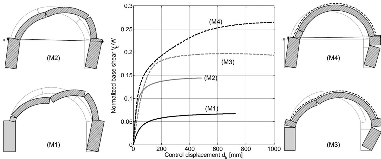
**Figure 7.** Push-over curves and failure mechanisms for arches on pillars with different strengthening devices: no strengthening (M1), tie-bar (M2), externally bonded composite material strips (M3), and tie-bar and externally bonded composite material strips (M4).
